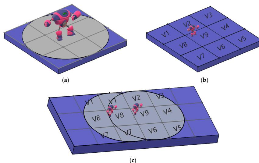
**Figure 1.** This figure displays the range of the sensor view in grid cells. Panel (a) shows the limited sensor range (V1 to V8) around the robot. Panel (b) shows the eight cells surrounding the robot, where cell 9 represents the robot's position. Panel (c) illustrates a scenario in which the robot moves from right to left, highlighting that the sensor range does not cover the cost values of V3, V4, and V5.
