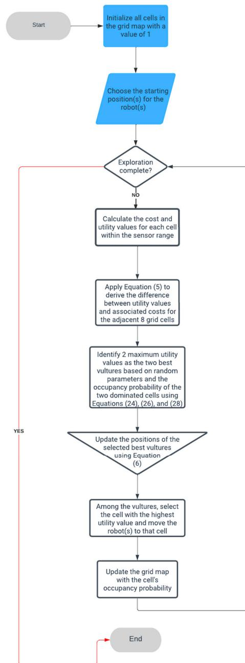
**Figure 2.** The hybrid optimization algorithm called Hybrid Vulture-Coordinated Multi-Robot Exploration HVCME.
