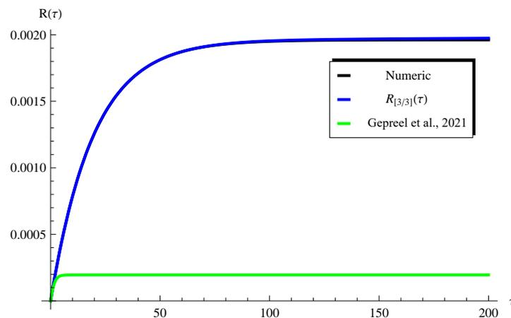
**Figure 16.** Comparison between the  $R_{[3/3]}(\tau)$  (present), the numerical solution, and the HPM (Ref. [23]) at  $A = 0$ ,  $B = 10^{-4}$ , and  $\sigma = 0.95$ .
