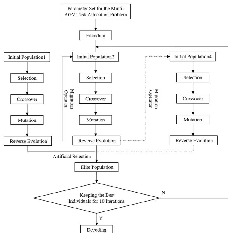
Figure 1. Flowchart of the Design Process for the Multi-Population Genetic Algorithm in this Study.
