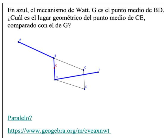
**Figure 1.** One of the tasks proposed to the students: *In blue, the Watt mechanism. G is the midpoint of BD. What is the locus of the midpoint of CE, compared to that of G?*
