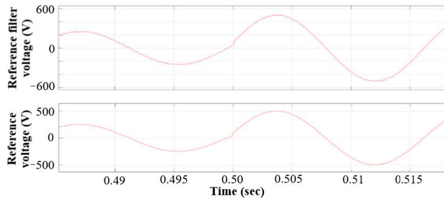
Figure 12. Dynamic response of FCS-MPC under frequency penalization.
