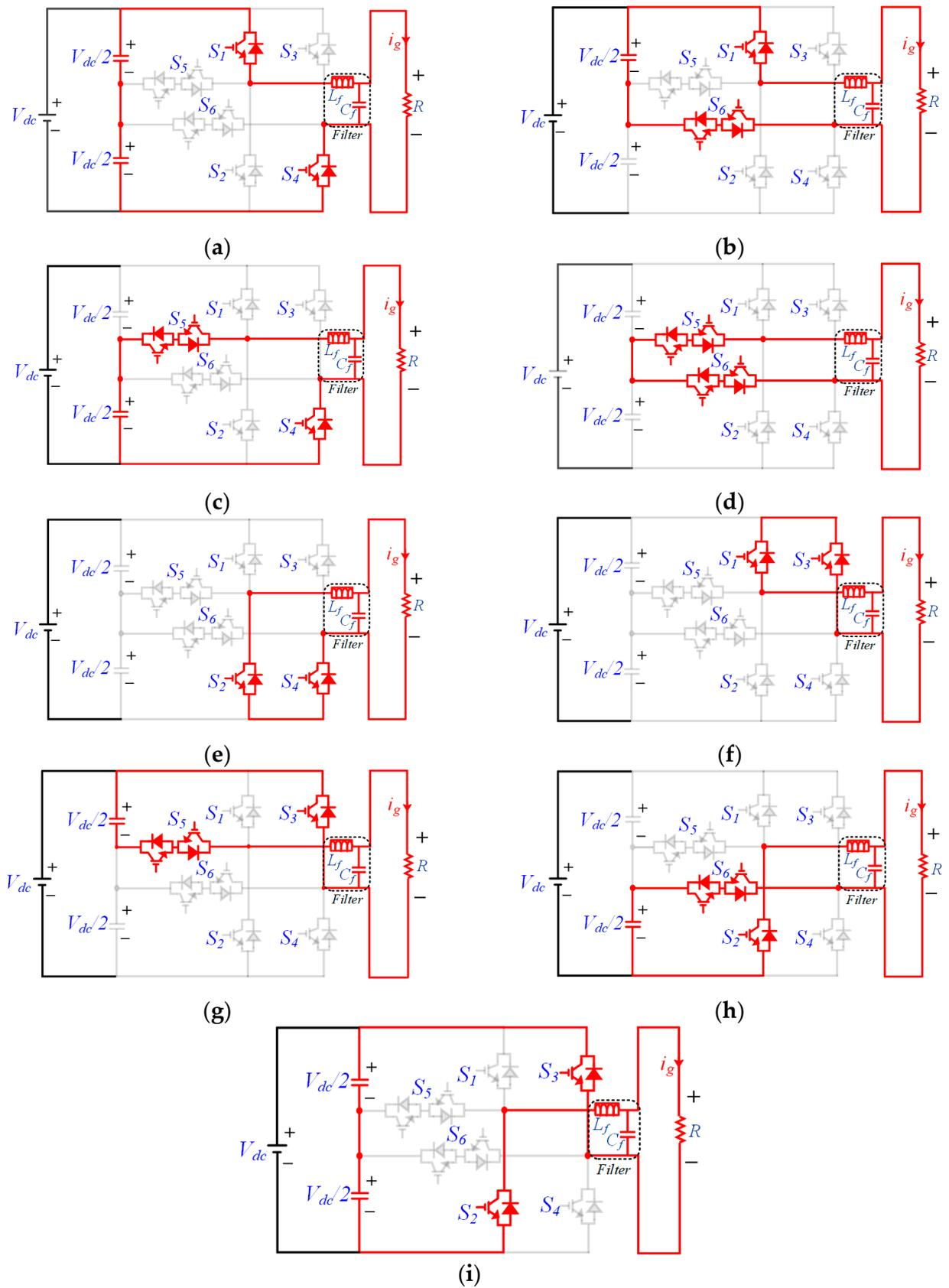
Figure 5. Different switching states of the topology. (a) T<sub>1</sub>; (b) T<sub>2</sub>; (c) T<sub>3</sub>; (d) T<sub>4</sub>; (e) T<sub>5</sub>; (f) T<sub>6</sub>; (g) T<sub>7</sub>; (h) T<sub>8</sub>; (i) T<sub>9</sub>.
