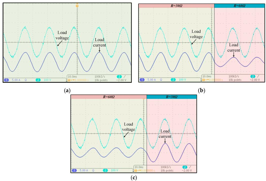
Figure 22. Output load voltage under dynamic loading conditions. Load voltage under different loading conditions. (a) Uniform load; (b) dynamic loading with load changing from  $R/2$  to  $R$ ; (c) dynamic loading with load changing from  $R$  to  $R/2$ .
