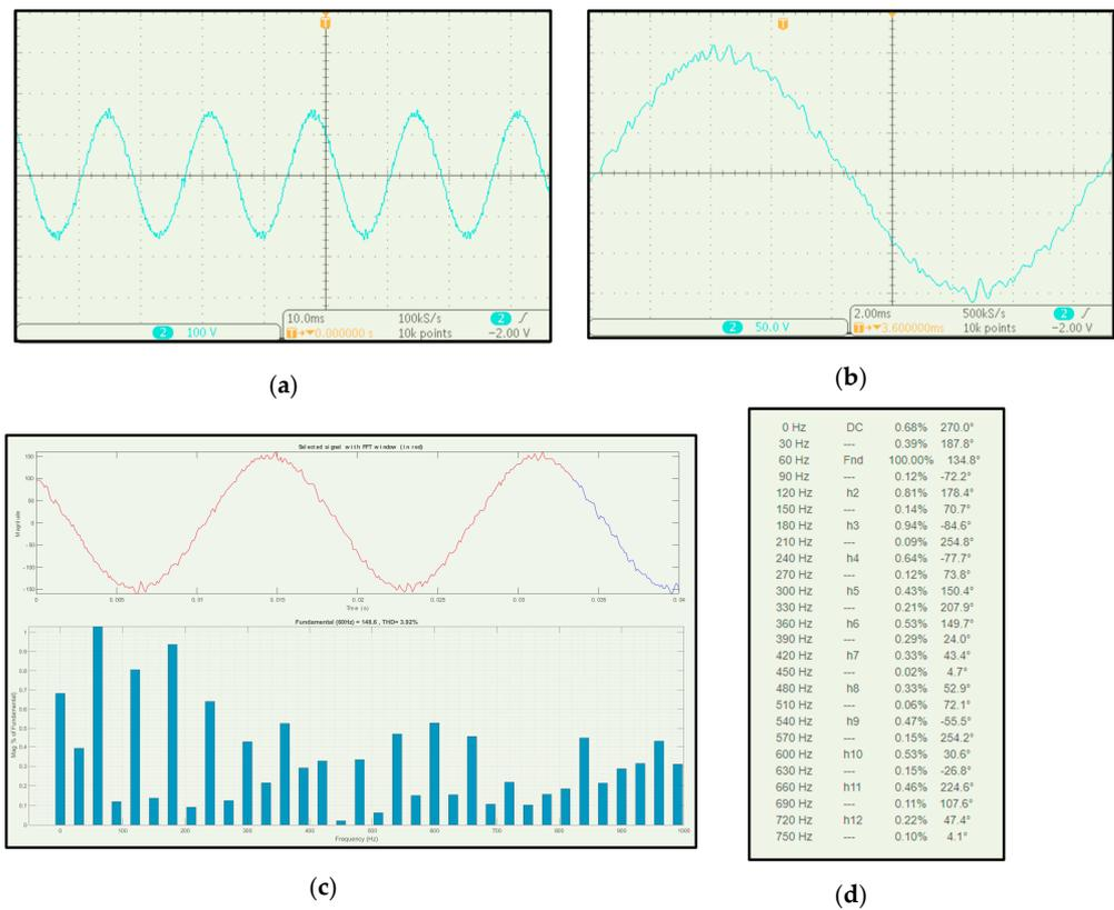
Figure 21. Load voltage. (a) With LC filter; (b) with LC filter (zoomed view); (c) with FFT spectrum; (d) harmonic content.
