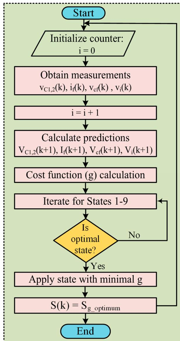
Figure 8. Flowchart of the FCS-MPC algorithm.
