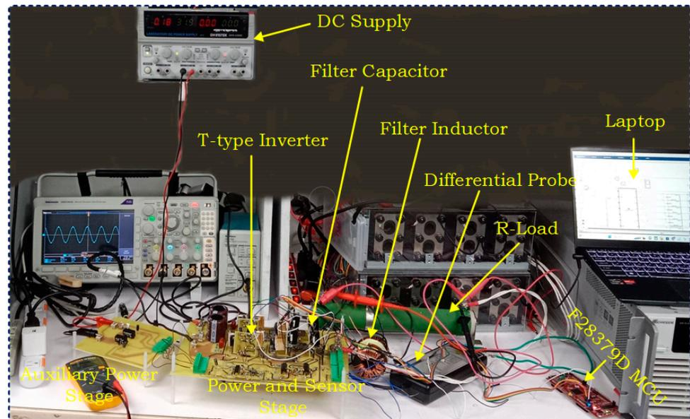
Figure 17. System test bench.
