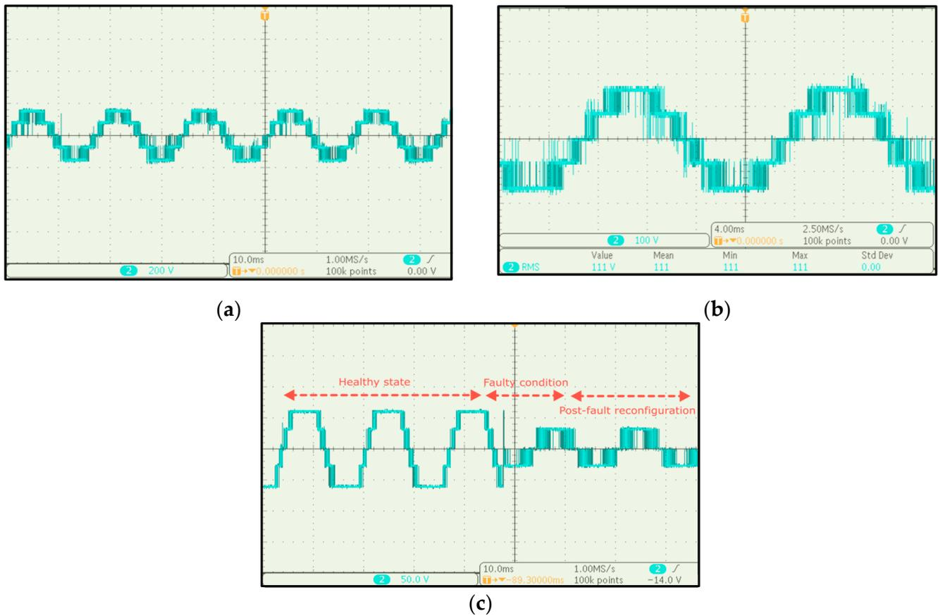
**Figure 20.** Inverter output voltage. (a) Without LC filter; (b) without LC filter (zoomed view); (c) post-fault transition.
