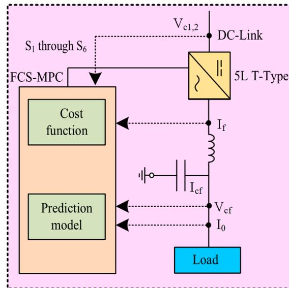
Figure 7. FCS-MPC and T-type system.
