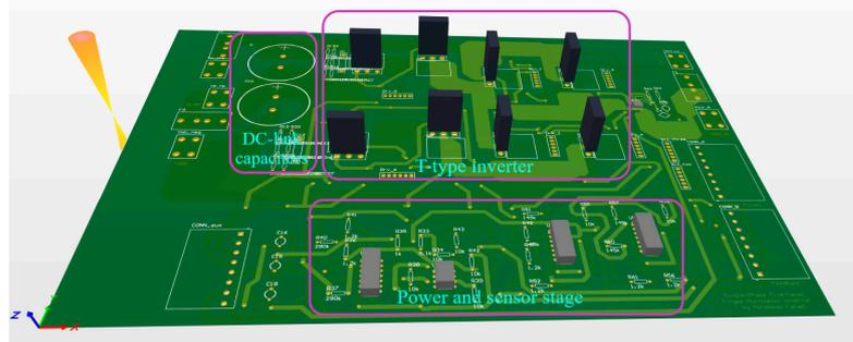
Figure 15. Power and sensor stage layout.
