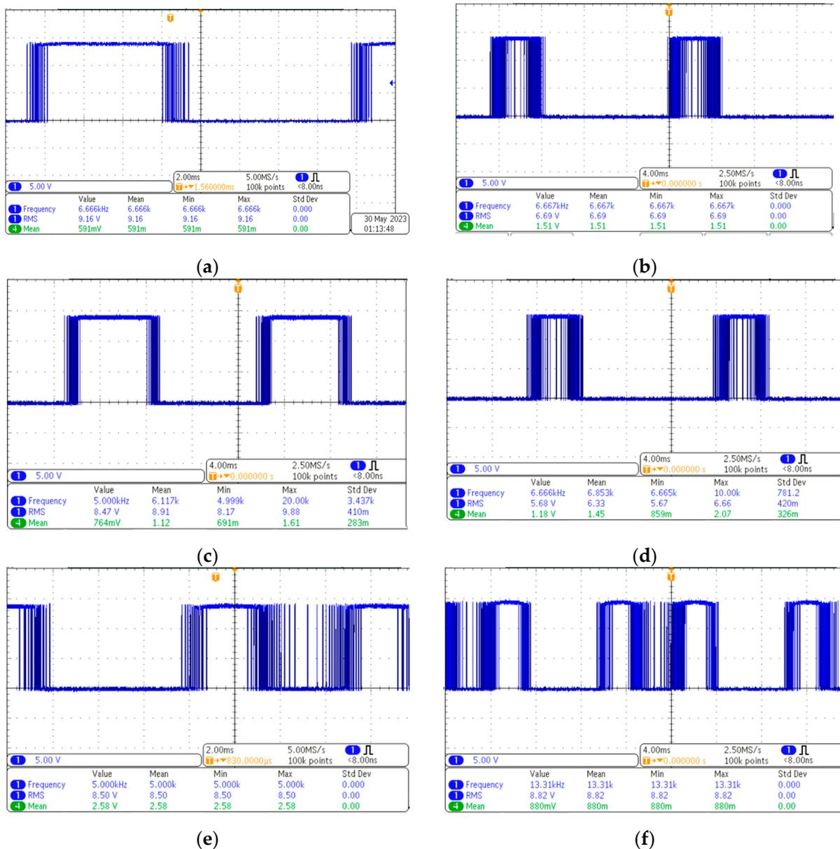
Figure 19. Switching signals to all the switches: (a)  $S_1$  gating; (b)  $S_2$  gating; (c)  $S_3$  gating; (d)  $S_4$  gating; (e)  $S_5$  gating; (f)  $S_6$  gating.
