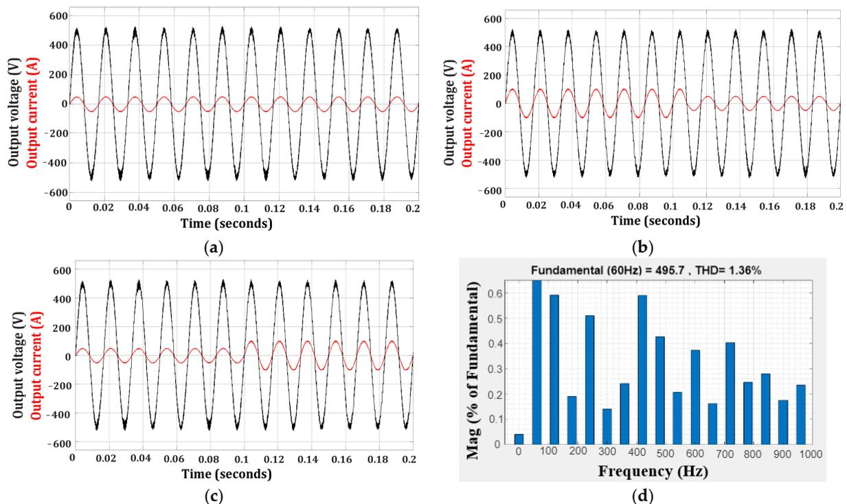
**Figure 13.** Load voltage under different loading conditions. (a) Uniform load; (b) dynamic loading with load changing from  $R/2$  to  $R$ ; (c) dynamic loading with load changing from  $R$  to  $R/2$ ; (d) harmonic profile of the output load voltage.
