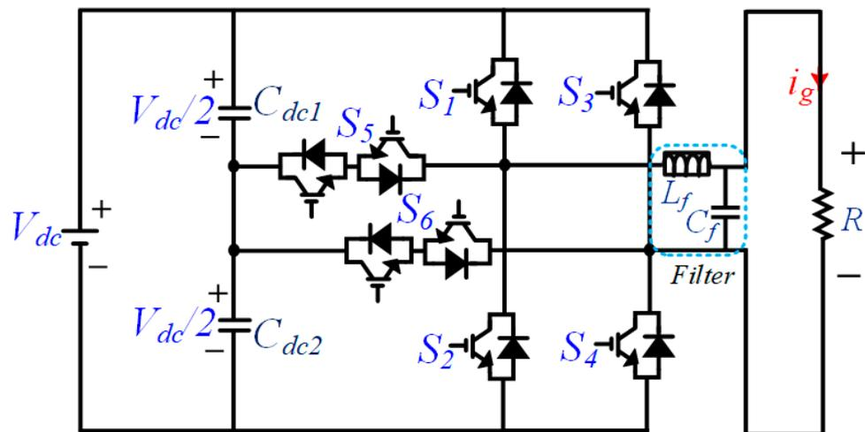
Figure 4. Single-phase five-level T-type topology structure.
