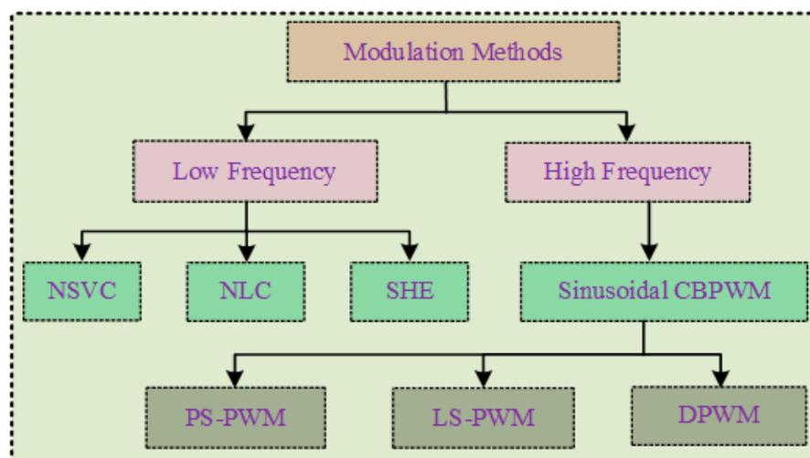
**Figure 2.** Modulation schemes for multilevel inverters.
