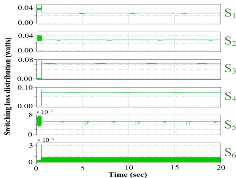
**Figure 9.** Switching loss distribution without penalization.
