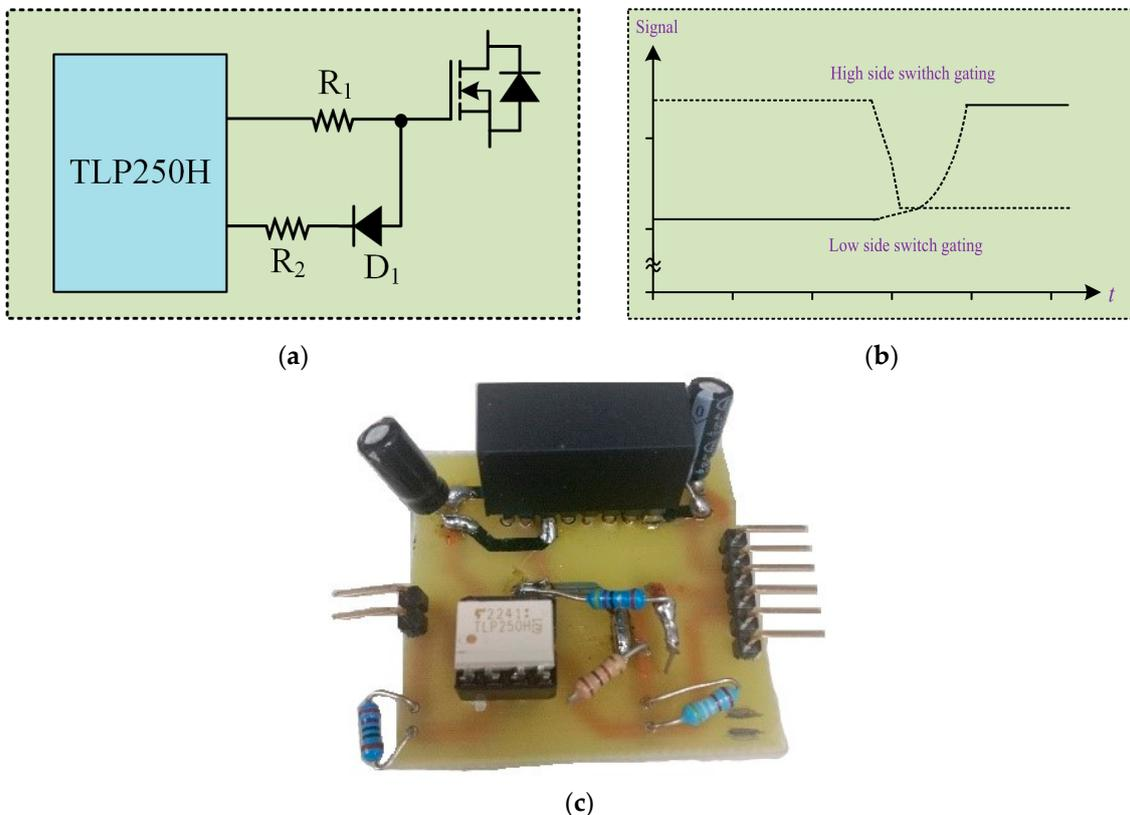
**Figure 14.** Hardware deadband implementation: (a) Block diagram representation; (b) deadband realization; (c) hardware of the gate driver unit.
