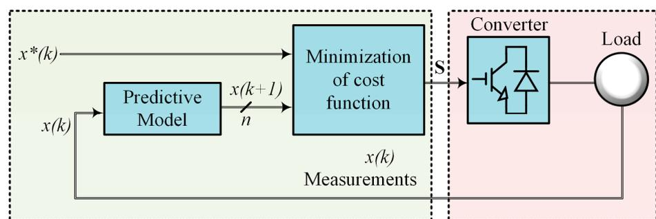
Figure 3. Block diagram of an FCS-MPC [21].
