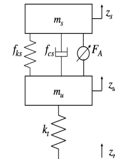
Figure 1. Quarter-Car Active Suspension System.
