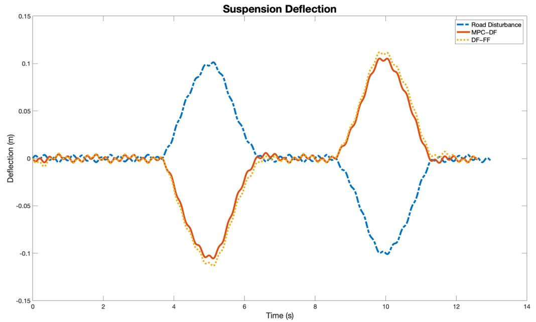
Figure 6. Suspension Deflection (Blue–Road Disturbance, Red–MPC-DF, Yellow–DF-FF).
