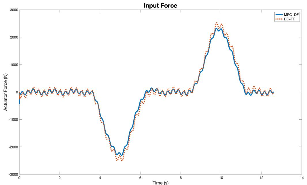
Figure 8. Input Force (Blue–MPC-DF, Red–DF-FF).
