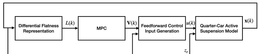
Figure 2. Block diagram of the proposed differential flatness-based Model Predictive Controller.
