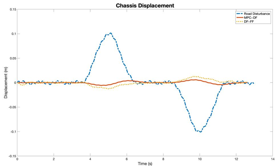
Figure 4. Chassis Displacement (Blue–Road Disturbance, Red–MPC-DF, Yellow–DF-FF).
