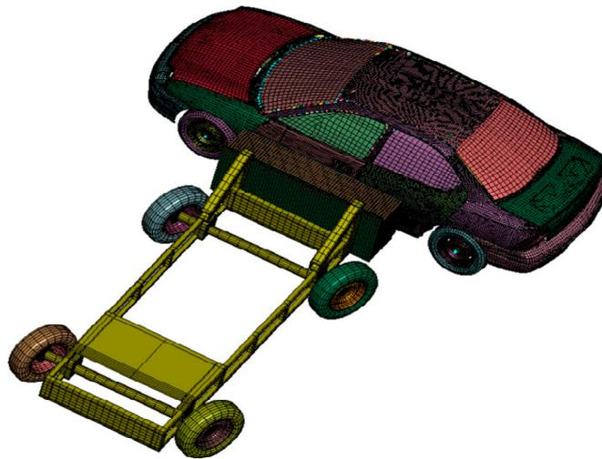
Figure 14. Three-dimensional model diagram of a car’s side crash.
