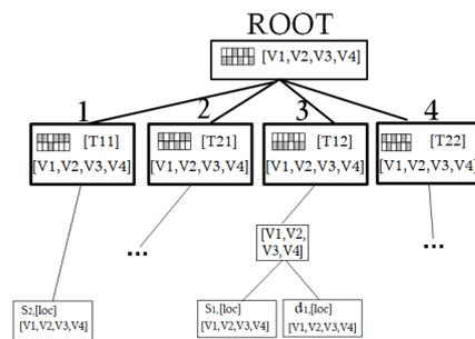
Figure 7. The structure of eRBFtree.  $[\cdot]$  is the encryption of  $\cdot$ .
