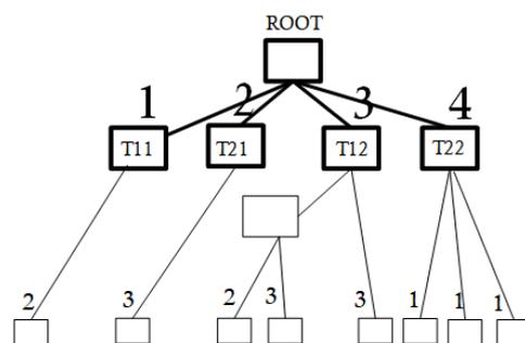
Figure 5. The quad tree structure for all points.
