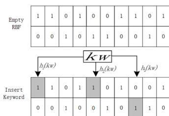
Figure 1. Inserting a keyword on an empty RBF.
