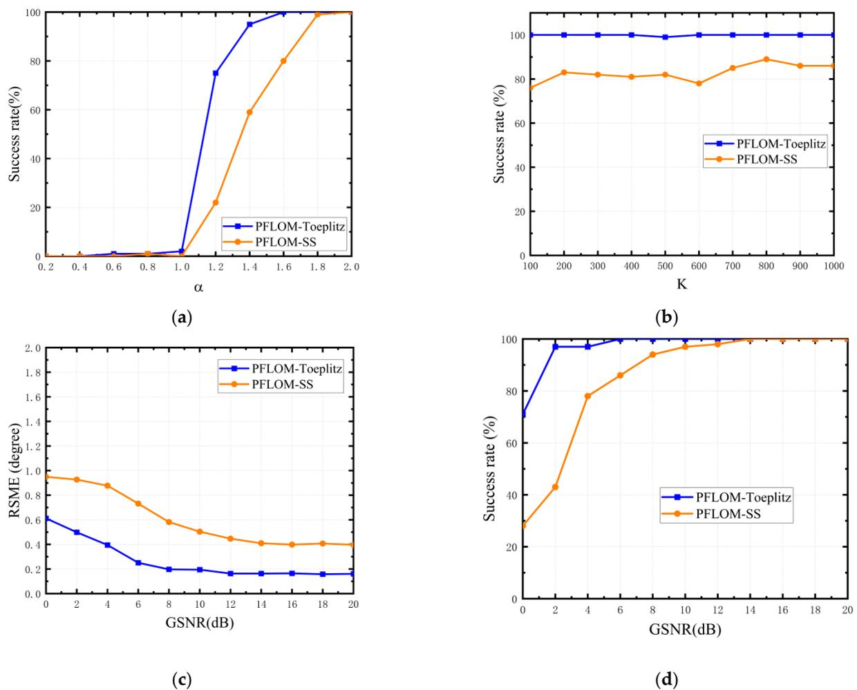
**Figure 6.** Performance comparison between PFLOM-SS and PFLOM-Toeplitz. (a) Estimated success rate versus  $\alpha$ . (b) Estimated success rate versus number of snapshots. (c) RMSE versus GSNR. (d) Estimated success rate versus GSNR.
