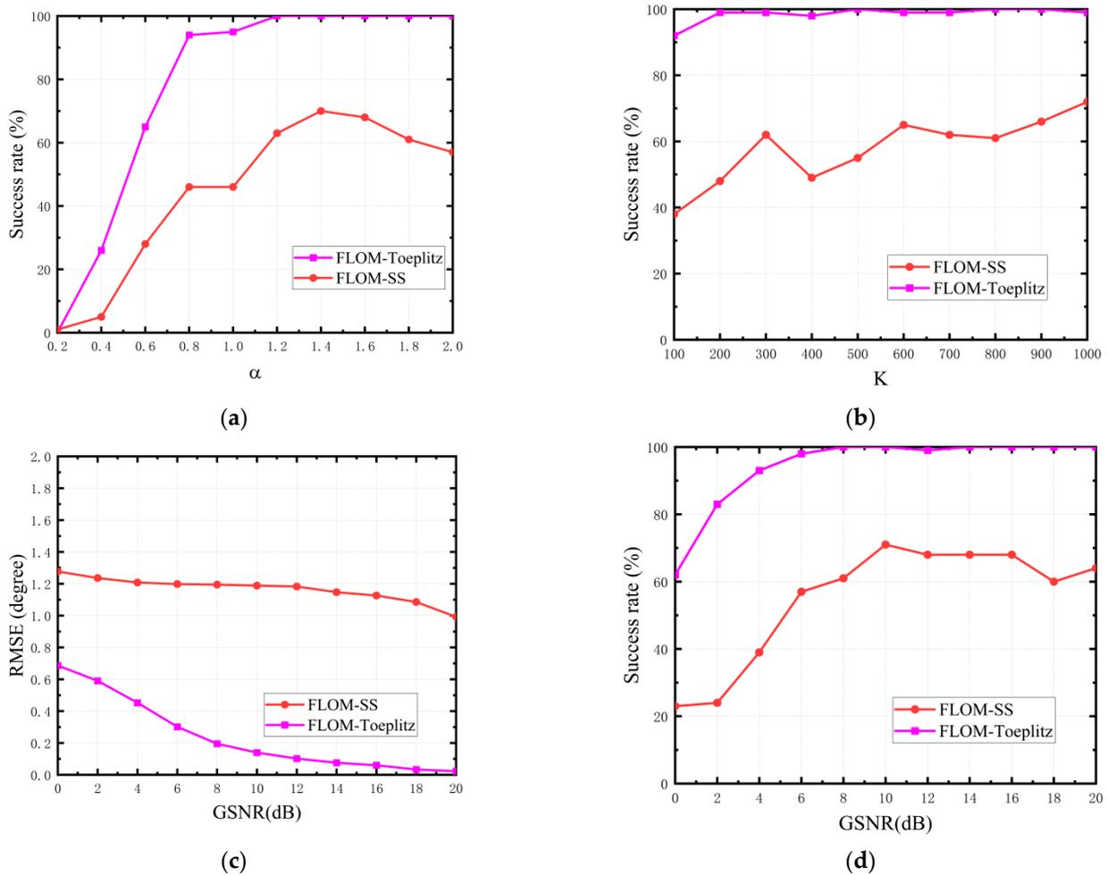
**Figure 5.** Performance comparison between FLOM-SS and FLOM-Toeplitz. (a) Estimated success rate versus  $\alpha$ . (b) Estimated success rate versus number of snapshots. (c) RMSE versus GSNR. (d) Estimated success rate versus GSNR.
