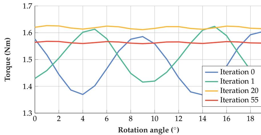
(b) Torque curves during optimization for robust optimization
