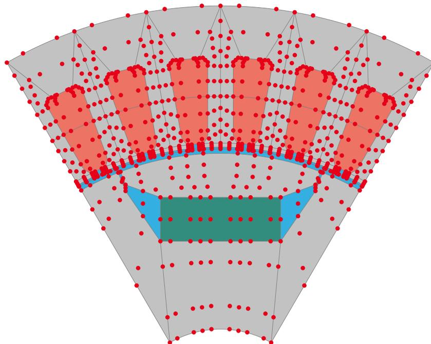
**Figure 2.** Geometry model of the PMSM with highlighted control points as described in (2) and patch boundaries. The model was originally based on [19].
