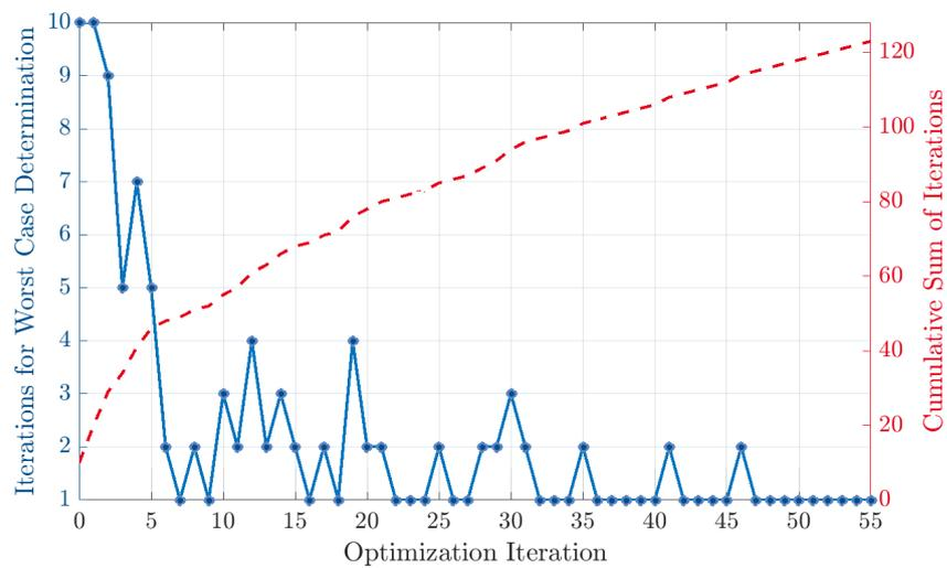
**Figure 6.** Number of iterations to determine the worst-case scenario during the robust optimization process. The number of needed iterations decreases with increasing optimization iterations.
