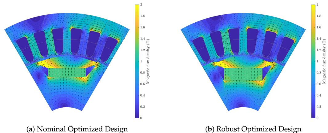
**Figure 7.** Resulting magnetic flux density of the the nominal design (a) and the robust design (b).
