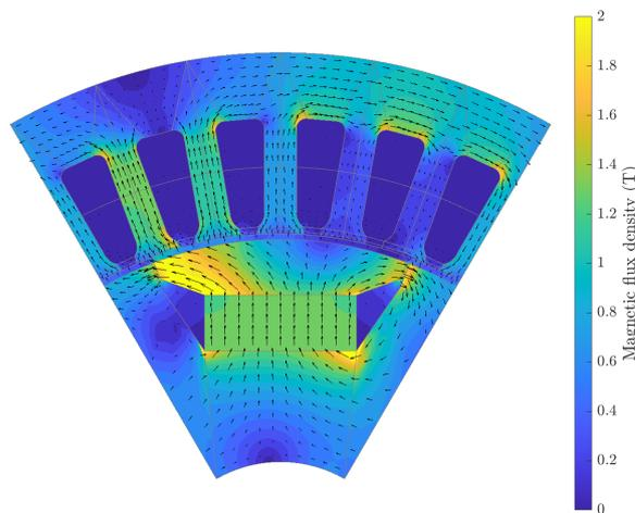
**Figure 3.** Plot of the solution to (9), representing the magnetic flux density.
