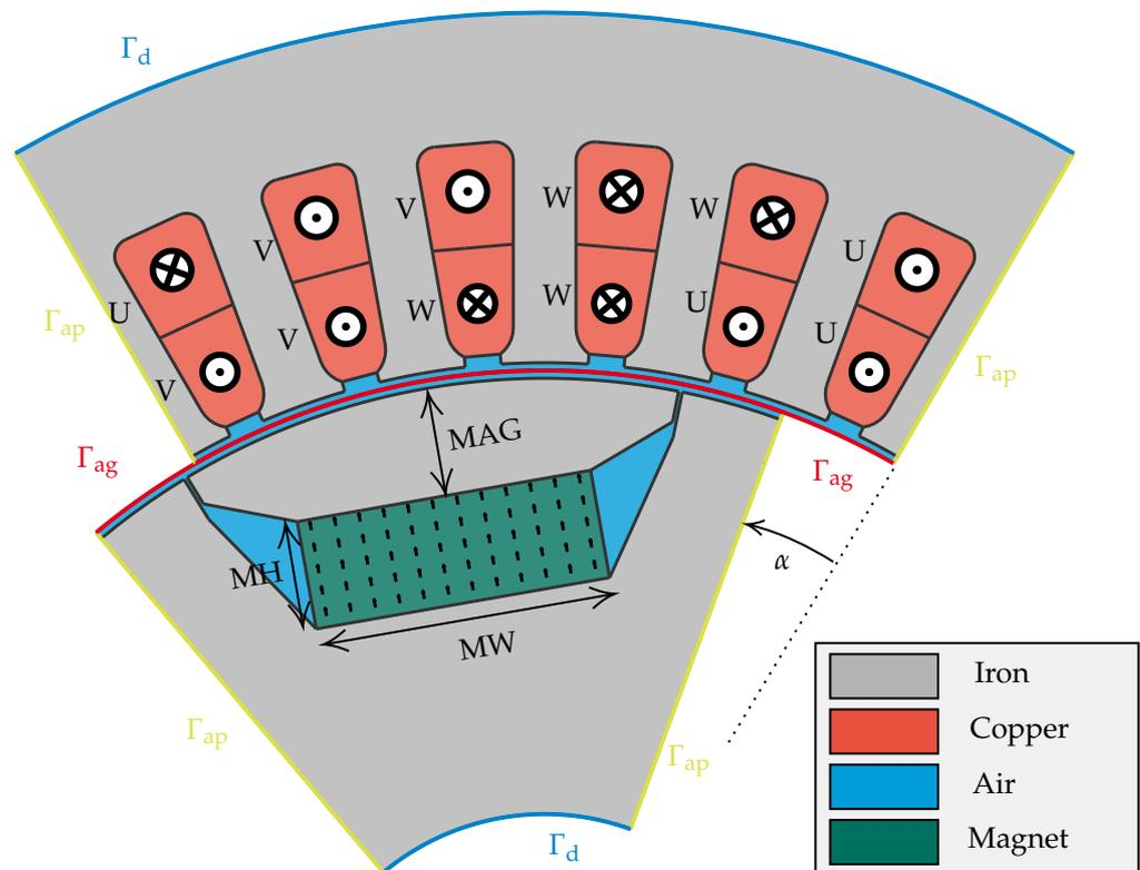
**Figure 1.** Geometry of 1/6 of a PMSM constructed in MATLAB® 9.14.0 R2023a using IGA and the open-source package GeoPDEs.
