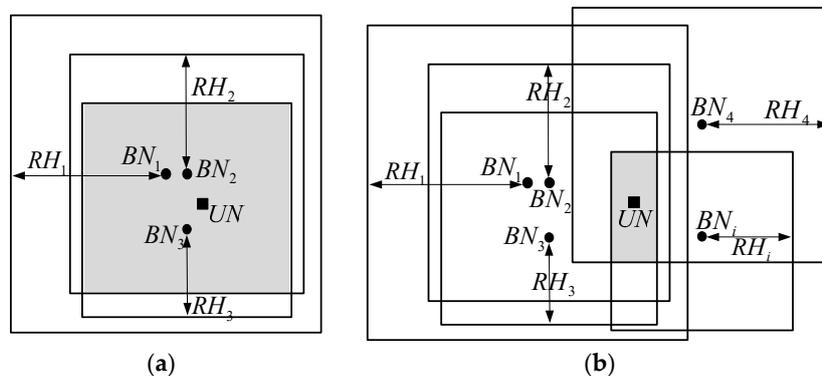
Figure 6. Population constraint strategy. (a) Population constraint based on three beacon nodes; (b) Population constraint based on all beacon nodes.
