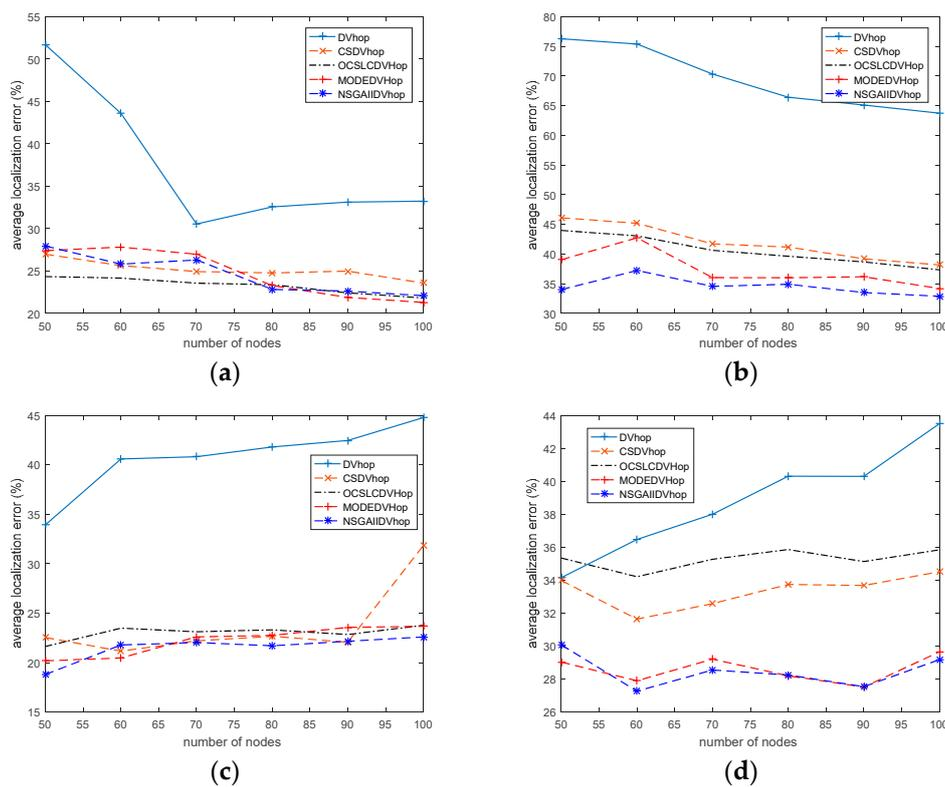
**Figure 10.** The ALE of four network topologies in different number of nodes. (a) The random topology; (b) The C-shaped random topology; (c) The O-shaped random topology; (d) The X-shaped random topology.
