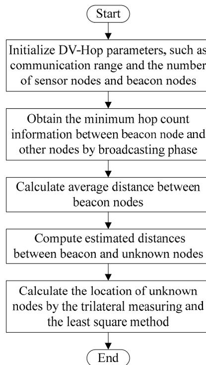
**Figure 1.** The distance vector-hop technique (DV-Hop) flowchart.
