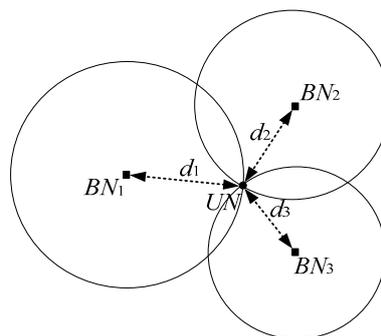
Figure 3. Constraint principle in ideal conditions.
