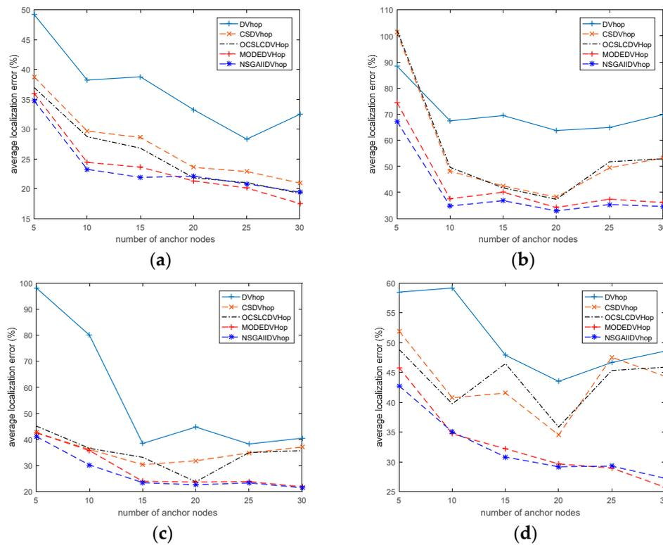
**Figure 11.** The ALE of four network topologies in different number of beacon nodes. (a) The random topology; (b) The C-shaped random topology; (c) The O-shaped random topology; (d) The X-shaped random topology.
