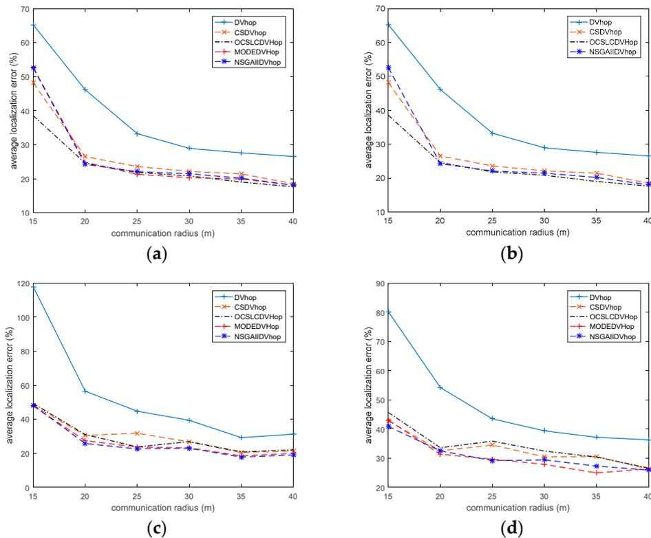
**Figure 9.** The ALE of four network topologies in different communication radius. (a) The random topology; (b) The C-shaped random topology; (c) The O-shaped random topology; (d) The X-shaped random topology.
