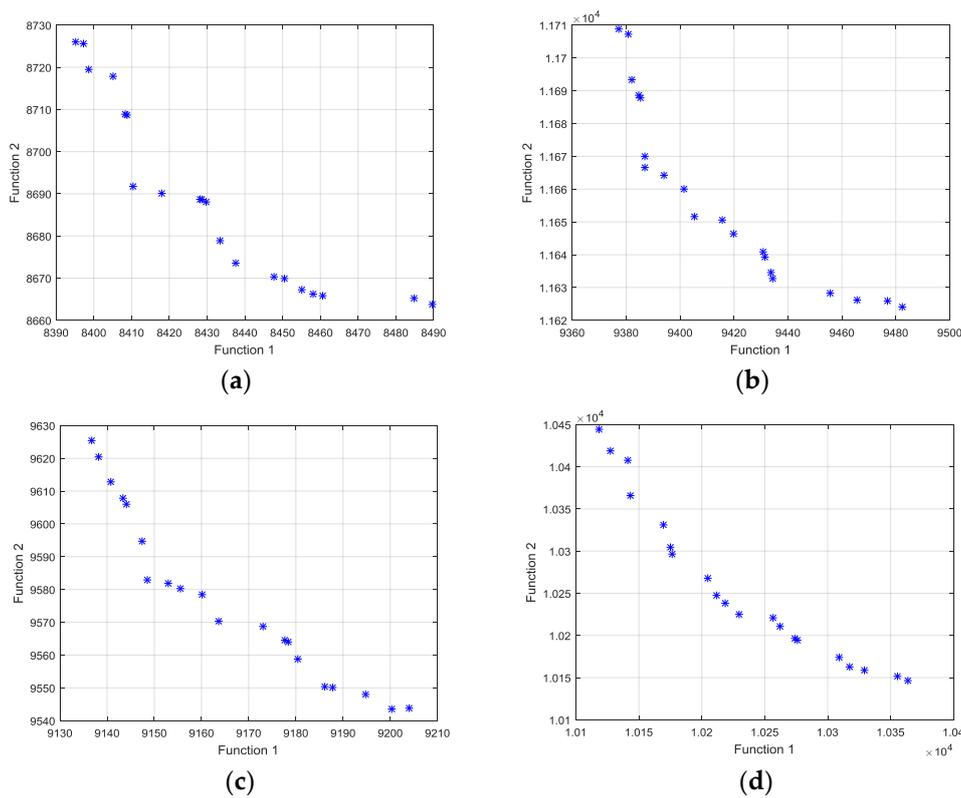
**Figure 8.** Two objective function relationships in four different network topologies. (a) The random topology; (b) The C-shaped random topology; (c) The O-shaped random topology; (d) The X-shaped random topology.
