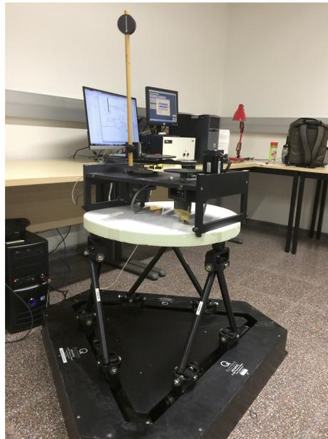
**Figure 1.** Experimental setup: Furuta pendulum located on a Stewart platform.
