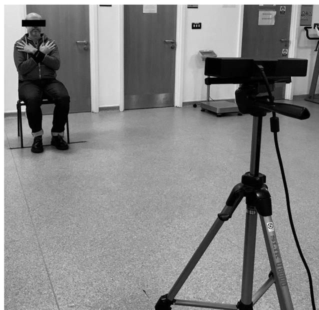
**Figure 2.** Example recording environment with the Microsoft Kinect One placed on a tripod at 70 cm.
