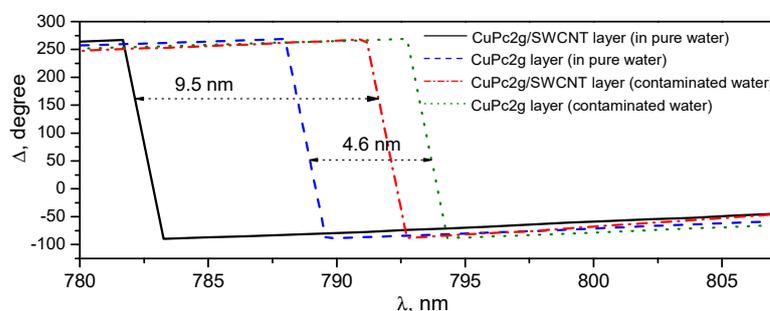
**Figure 18.**  $\Delta(\lambda)$  TIRE spectra of a CuPc2g film in water (dashed line), after injection of benzo[a]pyrene saturated solution (dotted line), and a layer of CuPc2g/SWCNT hybrid in water (solid line), after injection of benzo[a]pyrene saturated solution (dashed-dotted line).
