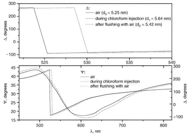
**Figure 13.**  $\Psi(\lambda)$  and  $\Delta(\lambda)$  TIRE spectra of CuPc3b-coated Cr/Au films. The effect of exposure to chloroform vapor. The enlarged section of the  $\Delta(\lambda)$  spectrum is shown above. Reprinted with permission from [44]. Copyright 2009, Elsevier.
