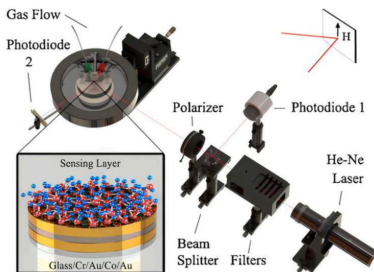
**Figure 9.** Experimental setup for SPR and MOSPR characterization in dry air and a controlled atmosphere. The magnetic field vector is represented; it is applied in the plane of the surface and perpendicular to the plane of incidence of light. Reprinted with permission from [55]. Copyright 2013 Elsevier.
