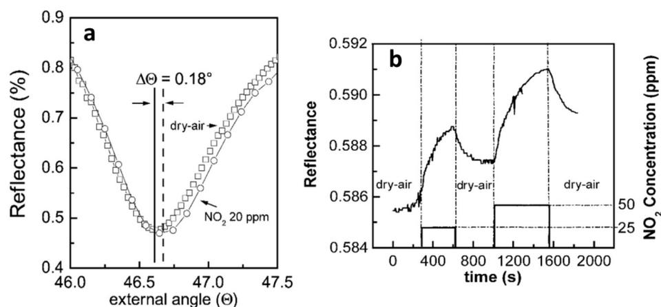
**Figure 21.** (a) SPR curves of a  $\text{TiO}_2/\text{FePc1a}$  layer in the presence of dry air flux and in ambient air containing 20 ppm  $\text{NO}_2$  gas. (b) Dynamic response measured in the presence of different concentrations of  $\text{NO}_2$  gas for a sol-gel  $\text{TiO}_2/\text{PdPc1a}$  film. Reprinted with permission from [97]. Copyright 2002, Elsevier.
