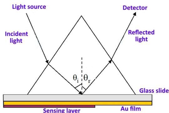
**Figure 2.** Kretschmann configuration used for SPR sensing.
