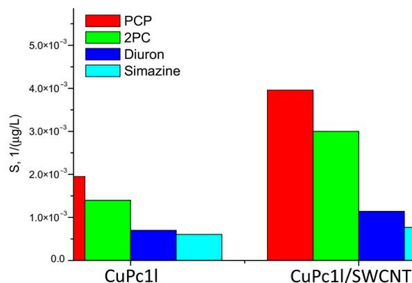
**Figure 19.** Sensitivity of CuPc1l and CuPc1l/SWCNT active layers to PCP, 2PC, diuron, and simazine. Reprinted with permission from [92]. Copyright 2016 Elsevier.
