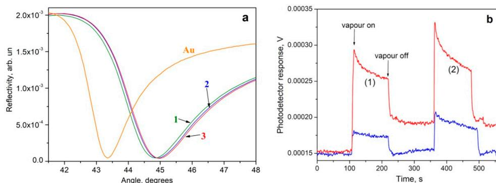
**Figure 7.** (a) SPR curves for a gold film (Au), initial gold/CuPc3b film (1), gold/CuPc3b film exposed to benzene (2), and chloroform (3). (b) Kinetics of the SPR response of CuPc3b films to chloroform (red line) and benzene (blue line) vapors of different concentrations: (1)  $p_s/10$ ; (2)  $p_s/5$  ( $p_s$  is the saturated vapor pressure). Reprinted with permission from [44]. Copyright 2009, Elsevier.
