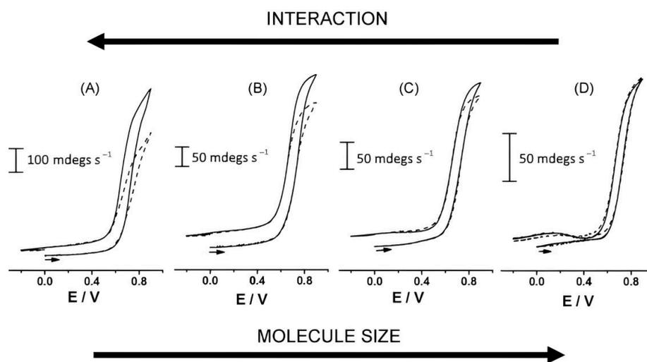
**Figure 16.** Dependence of the SPR reflection angle on the applied potential at a Por5/Au interface in pure 0.1 M NaClO<sub>4</sub> electrolyte solution (dashed line) and in the presence of 100 M (solid lines) of (A) catechol, (B) dopamine, (C) acetaminophen, and (D) ferrocyanide. Reprinted with permission from [76]. Copyright 2009, Elsevier.
