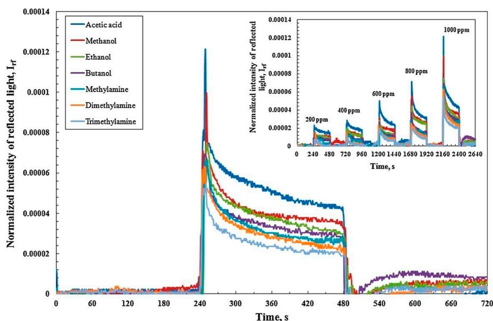
**Figure 6.** SPR sensor response of FAIPc spun films to various VOCs (1000 ppm) (inset: the response to five different vapor concentrations). Reprinted with permission from [43]. Copyright 2016 Elsevier.
