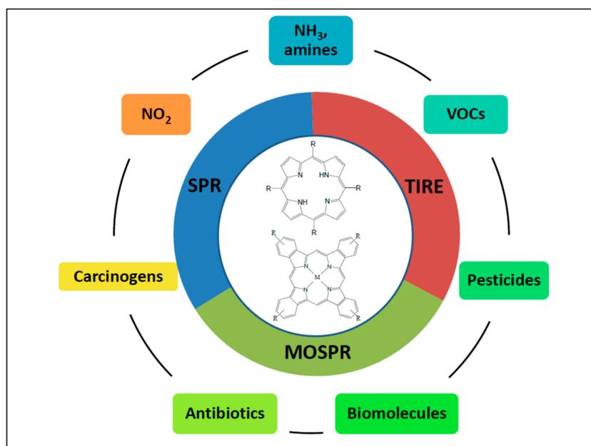
**Figure 1.** Scheme showing the use of optical sensors based on the phenomenon of plasmon resonance, using metal phthalocyanines and porphyrin derivatives as active layers.
