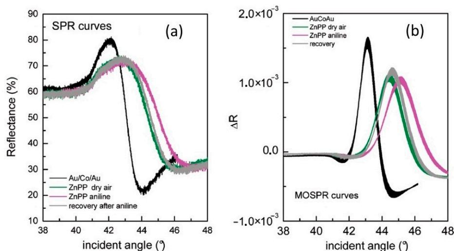
**Figure 11.** SPR (a) and magneto-optical (b) curves showing the change in optical features of the Au/Co/Au multilayer after deposition of the ZnPP LS thin films and after its interaction with saturated aniline vapors. Recovery of the sensing surface is also evidenced. Reprinted with permission from [21]. Copyright 2012, American Chemical Society.
