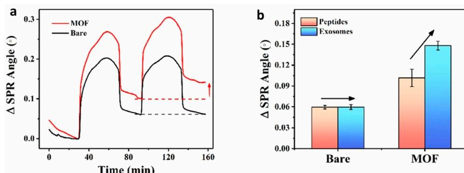
**Figure 23.** SPR raw signal (a) and data analysis (b) of peptides and exosomes flowed through the bare gold chip and 2D MOF chip, respectively. Reprinted with permission from [106]. Copyright 2022 Elsevier.
