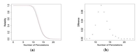
**Figure 16.** (a)  $R^{H_{7\times 5}}(x)$  calculated using our algorithm when the electrical current can move in all directions (top curve) and when movement is restricted (bottom curve) when  $p_1 = 0.98$  and  $\beta = 0.005$  and (b) the difference between the  $R^{H_{7\times 5}}(x)$ .
