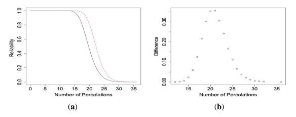
**Figure 12.** (a)  $R^{H_{g}} \times g(x)$  calculated using our algorithm when the electrical current can move in all directions (top curve) and when movement is restricted (bottom curve) when p = 0.90 and (b) the difference between the  $R^{H_{g}} \times g(x)$ .
