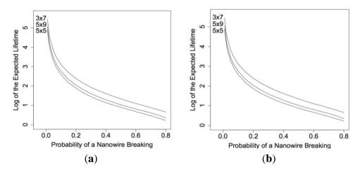
**Figure 6.**  $log E(X_{n \times m}^{H})$  calculated using our algorithm for various values of *n* and *m* when (a) the electrical current can move in all directions and when (b) movement is restricted.
