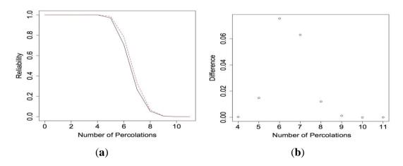
We can also show that a significant increase in reliability occurs for nanosensors with ETL and HL structures of larger sizes. Figure 11a shows the reliability functions for a  $21 \times 21$  nanosensor with ETL structure when p = 0.95, and Figure 12a shows the reliability functions for a  $9 \times 9$  nanosensor with HL structure when p = 0.90. For both figures the dashed lines represent the reliability when the electrical current can move in all directions.
