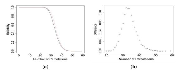
**Figure 11.** (a)  $R^{E}_{21 \times 21}(x)$  calculated using our algorithm when the electrical current can move in all directions (top curve) and when movement is restricted (bottom curve) when p = 0.95 and (b) the difference between the  $R^{E}_{21 \times 21}(x)$ .
