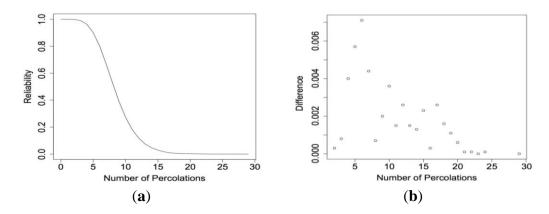
**Figure 15.** (a)  $R_{7 \times 13}^{E}(x)$  calculated using our algorithm when the electrical current can move in all directions (top curve) and when movement is restricted (bottom curve) when  $p_1 = 0.95$  and  $\beta = 0.01$  and (b) the difference between the  $R_{7 \times 13}^{E}(x)$ .
