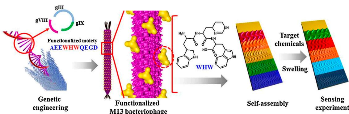
**Figure 9.** Scheme of phage-based colorimetric sensor preparation. M13 bacteriophages are engineered to display WHW ( $\pi$  aromatic interacting motif) on their pVIII major coat proteins. Subsequently, phages are pulled on the carrier to form a self-assembled structure [94]. Reprinted from [94], Copyright 2017, with permission from Elsevier.
