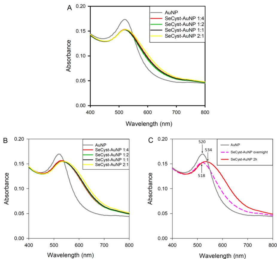
**Figure S9.** UV-vis spectra of A) SeCyst-AuNP after 2 h incubation, and B) SeCyst-AuNP after overnight incubation in HEPES buffer adjusted at pH 7.4, at the various ratios. C) Comparison of the UV-vis spectrum of SeCyst-AuNP after 2 h (dashed line), and SeCyst-AuNP overnight (bold line).
