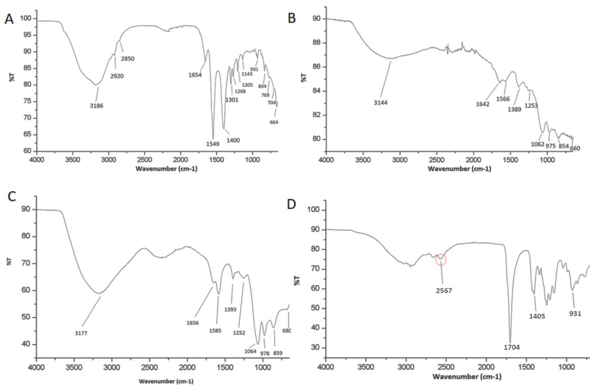
**Figure S13.** ATR-FTIR spectra of A) 3-MPA solution (pH 10.95), B) 3-MPA-AuNP purchased, C) 3-MPA-AuNP synthesized, and D) 3-MPA solution (pH 4.1).
