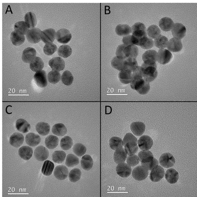
**Figure S16.** TEM micrograph of A) Cit-AuNPs, B) Cys-AuNPs, C) 3-MPA-AuNPs, and D) SeCyst-AuNPs using the synthesized AuNPs.
