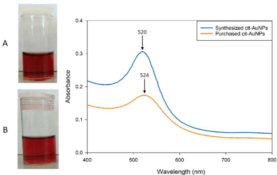
**Figure S1.** Comparison of colloidal solutions and UV-vis extinction spectra of citrate stabilized AuNPs, A) synthesized solution with absorbance maximum at 520 nm, and B) purchased solution with a maximum at 524 nm.
