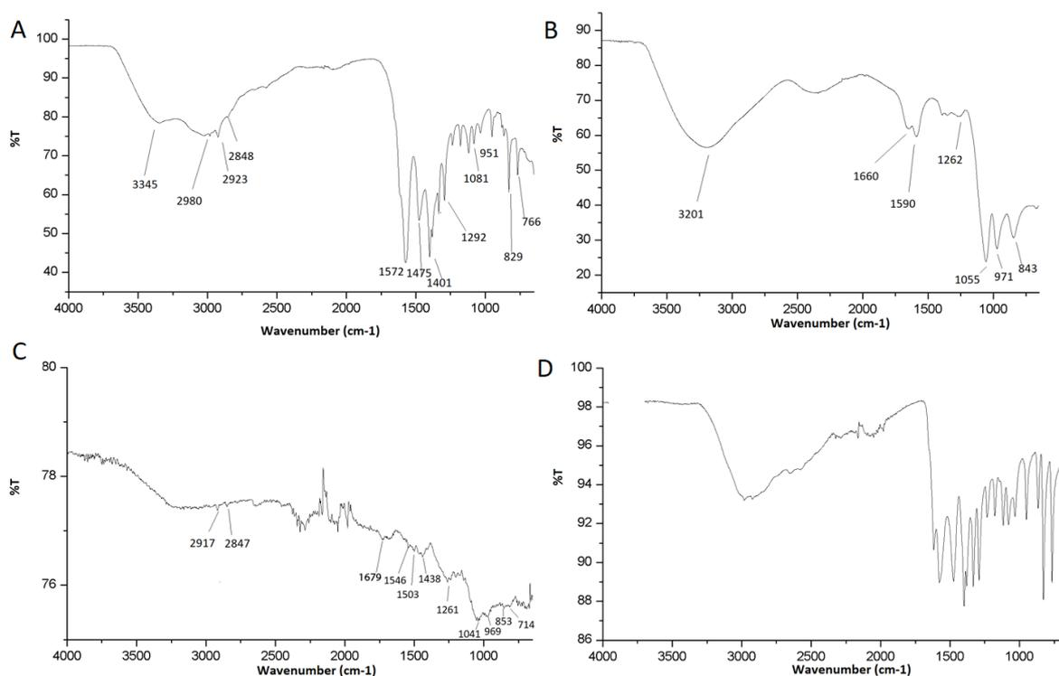
**Figure S14.** ATR-FTIR spectra of A) L-selenocystine solution (pH 10.20), B) SeCyst-AuNP synthesized, C) SeCyst-AuNP purchased, and D) L-selenocystine solution (pH 9.0).
