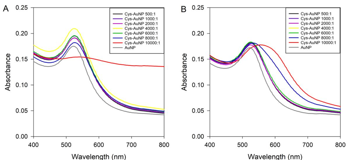
**Figure S19.** UV-vis spectra for stability assessment of Cys-AuNPs A) in D<sub>2</sub>O, and B) in deionized water at high concentrations (0.256-5.06 M).
