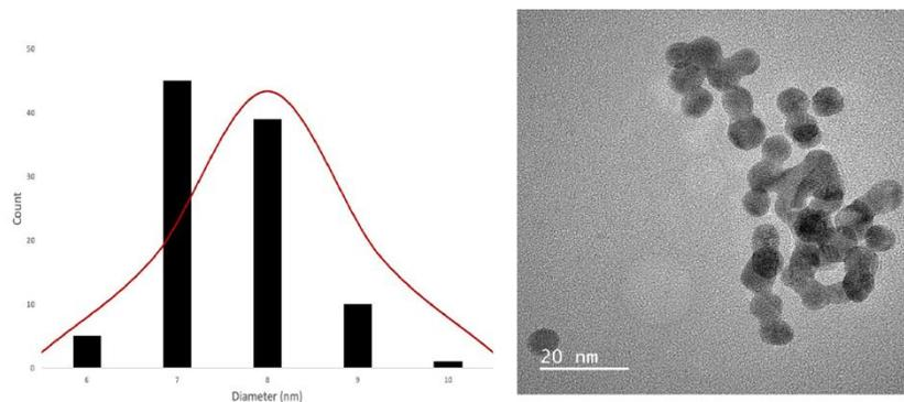
**Figure S2.** Histogram of the particle diameter of purchased Cit-AuNPs. The average diameter was calculated for 100 nanoparticles using ImageJ software.
