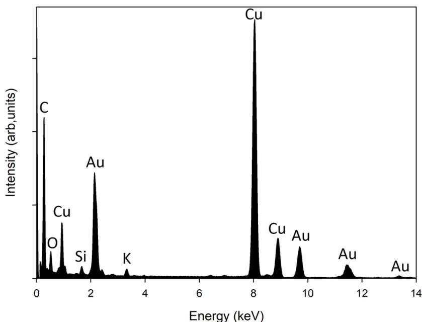
**Figure S17.** EDX spectrum from the analyzed area of the synthesized AuNPs with the Au  $M\alpha$  signals identified (C, O, Si and Cu may be from the supporting TEM grid and carbon film, while K signal may be from external contamination).
