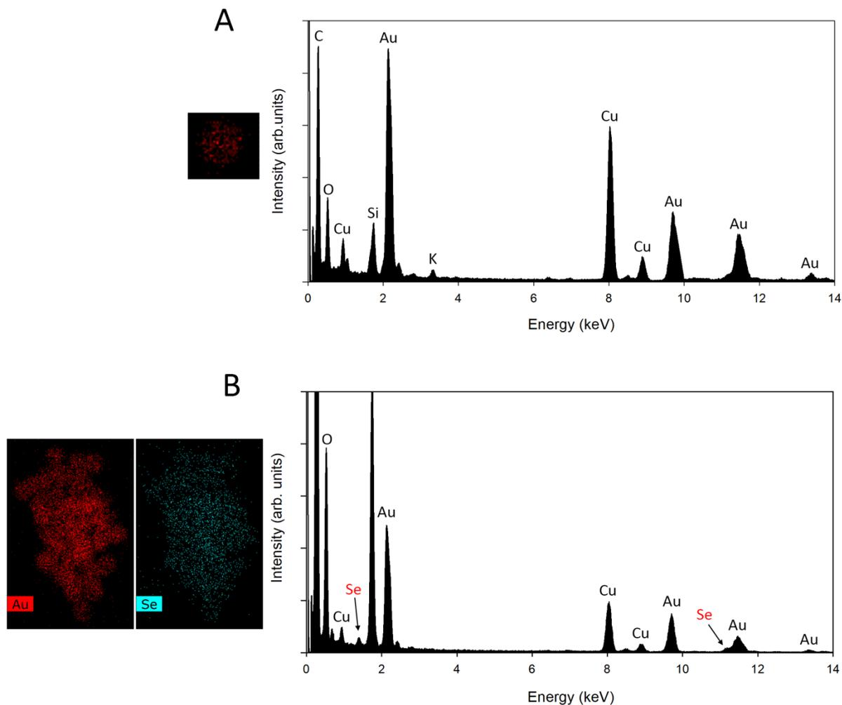
**Figure S18.** Analysis of SeCyst-AuNPs using the purchased nanoparticles, confirming the successful functionalization with SeCyst. A) Au EDX map on the left side and EDX spectrum of the purchased AuNPs. B) Au and Se EDX map on the left side and EDX spectrum from the analyzed area, with both  $M\alpha$  and  $Se\ L\alpha$  signals (C, O, Si and Cu may be from the supporting TEM grid and carbon film).
