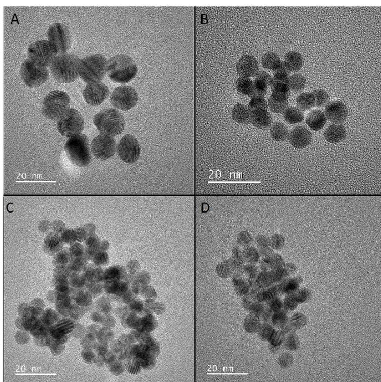
**Figure S15.** TEM micrograph of A) Cit-AuNPs, B) Cys-AuNPs, C) 3-MPA-AuNPs, and D) SeCyst-AuNPs using purchased nanoparticles.
