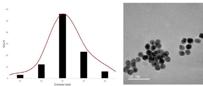
**Figure S3.** Histogram of the particle diameter of synthesized Cit-AuNPs. The average diameter was calculated for 100 nanoparticles using ImageJ software.
