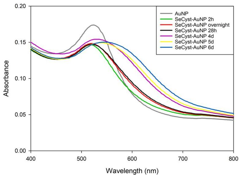
**Figure S10.** UV-vis spectrum of SeCyst-AuNP (1:2 ratio) in phosphate buffer pH 7.7 over a period of 6 days.
