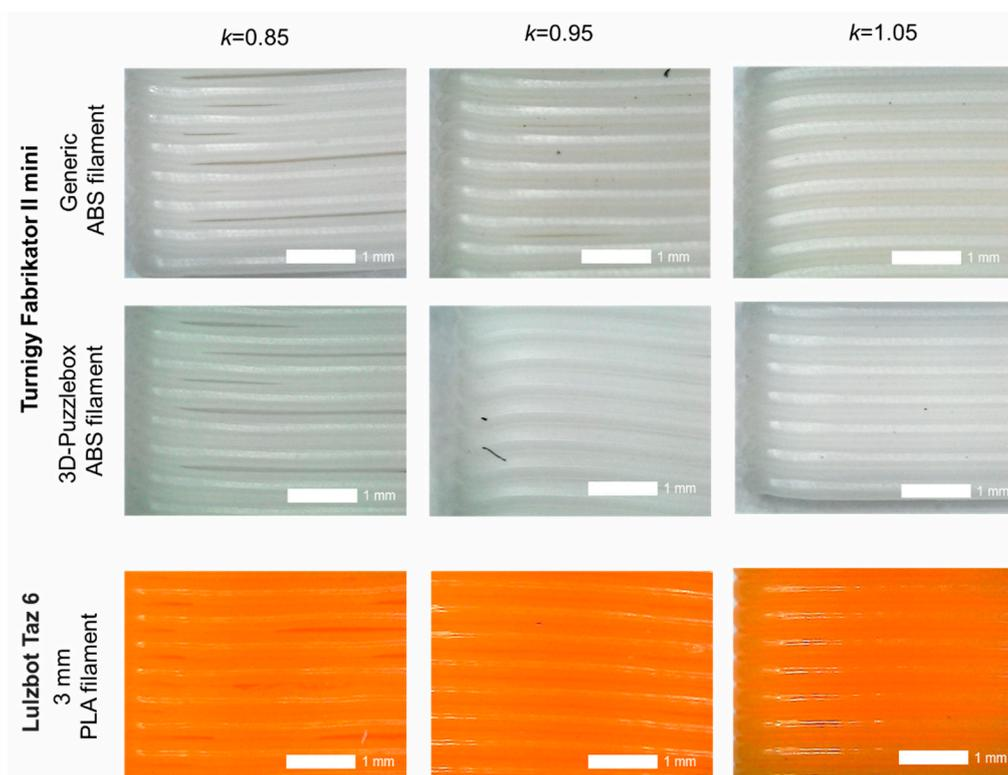
**Figure S2.** Optical microscope images of 3D-printed junctions fabricated with 0.40 mm layer height and extrusion ratios  $k=0.85$ , 0.95, or 1.05 using different 3D-printers and polymer filaments.
