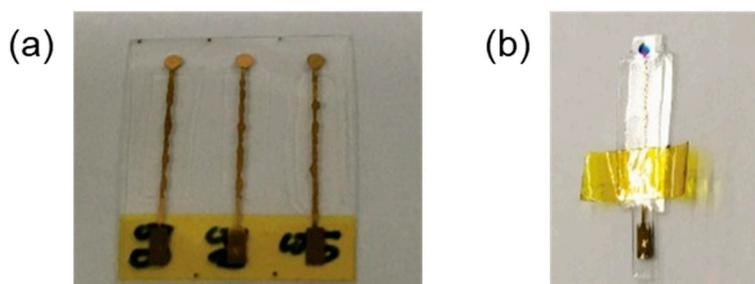
**Figure S1.** Photographs of inkjet-printed gold electrodes (a) before and (b) after IrO<sub>x</sub> electrodeposition.
