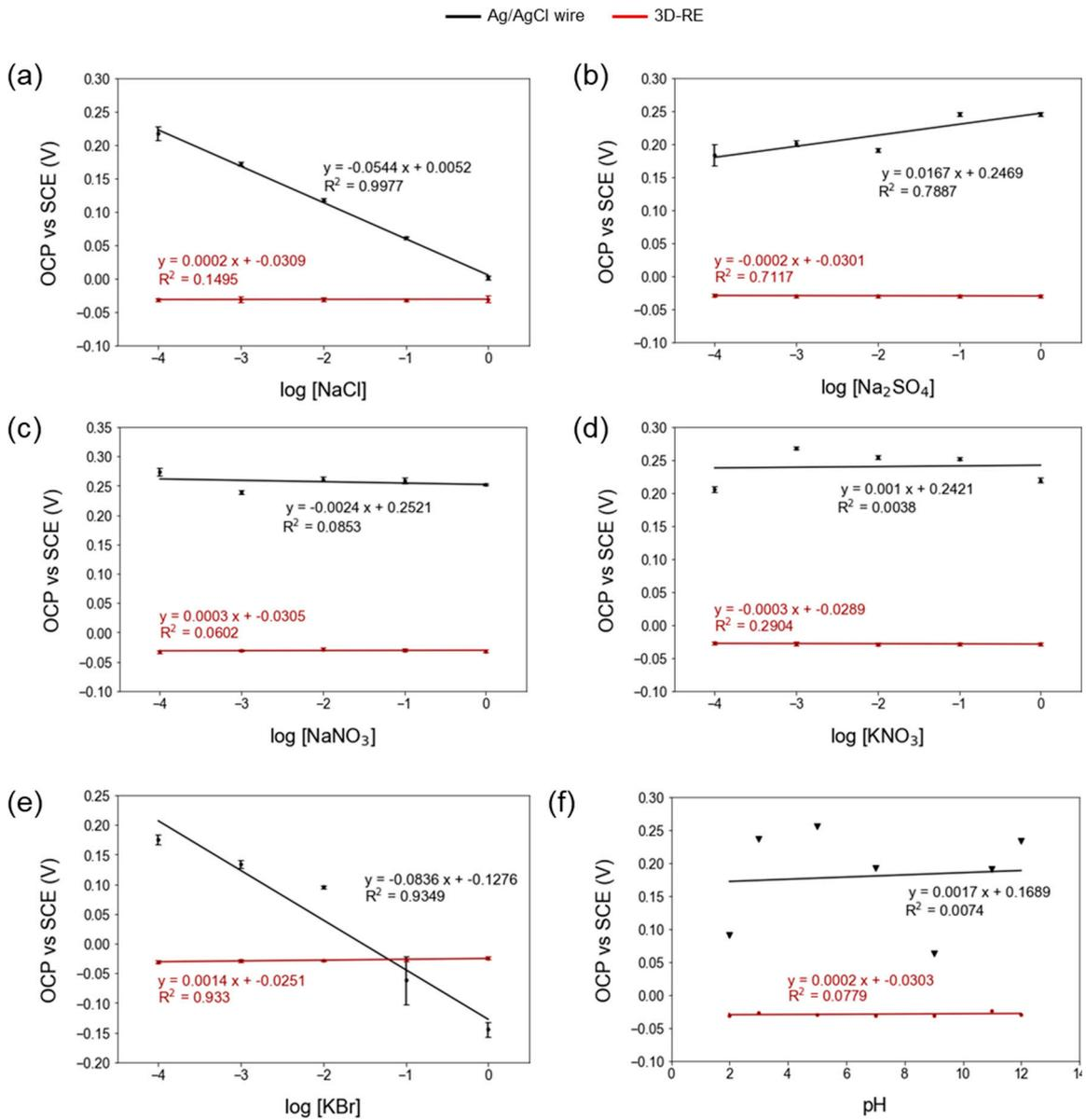
**Figure S4.** Nernst plots showing Ag|AgCl pseudoreference electrode and 3D-RE OCP dependence on the logarithm of concentration of different electrolytes or pH conditions. Error bars represent standard deviation.
