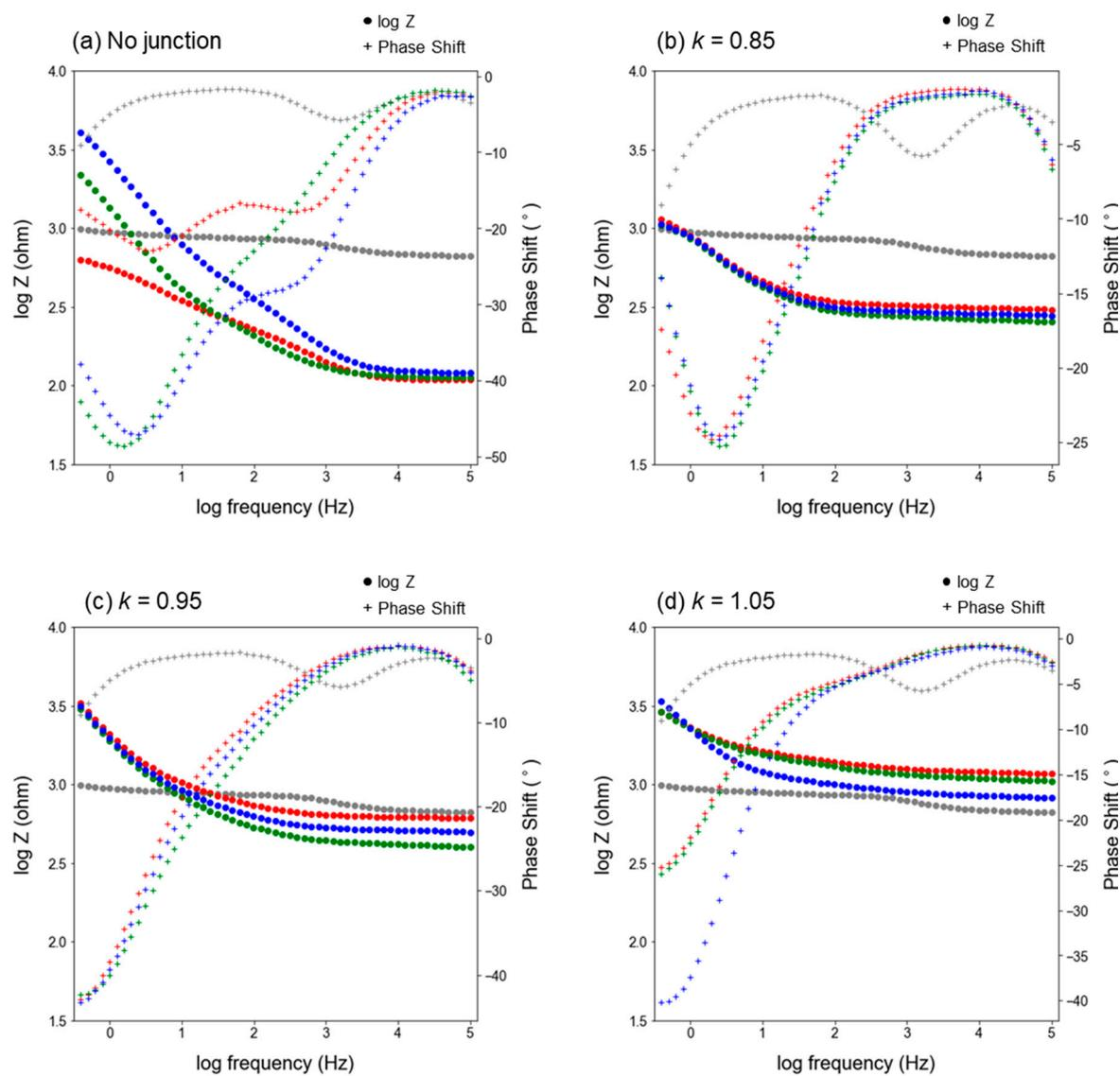
**Figure S3.** Bode plots of 3D-REs fabricated in three different batches (each replicate shown in either red, green, or blue) with (a) no junction, (b) 3D-printed junction with  $k = 0.85$ , (c) 3D-printed junction with  $k = 0.95$ , and (d) 3D-printed junction with  $k = 1.05$ . For reference, the bode plot of a commercial SCE (in grey) is also included in each plot. Impedance spectra were recorded in 0.1 M KCl.
