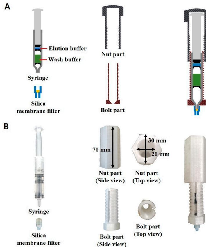
**Figure 1.** Syringe-based one-step DNA extraction device. (A) Schematic illustration of each component of the syringe-based DNA extraction device. The elution buffer and wash buffer fill the syringe, compartmentalized with the inverted bowl-shaped rubber packing. (B) Photographs of each component of the syringe-based DNA extraction device.
