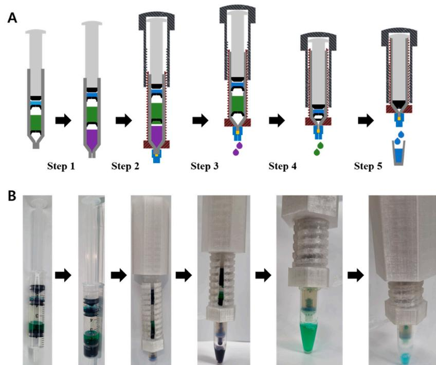
**Figure 2.** Operation procedure of the syringe-based one-step DNA extraction device. (A) Schematic illustration of the DNA extraction procedure using the syringe-based DNA extraction device. (B) Photographs of the syringe-based DNA extraction device at each step of the extraction procedure.
