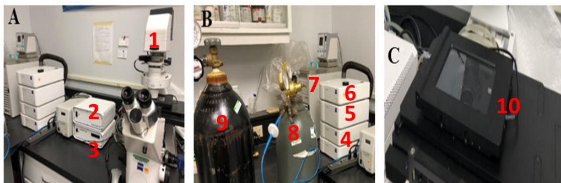
Scheme S3. Setup for the epifluorescence microscope. The components are labeled as 1. Zeiss Axio Observer (CAN-BUS) inverted microscope, 2. Power Supply, 3. Definite Focus module, 4. Temperature module, 5. CO 2 module, 6. O 2 module, 7. Heating device/humidity, 8. 100% CO 2 cylinder, 9. 100% N 2 cylinder, 10. Incubator chamber.
