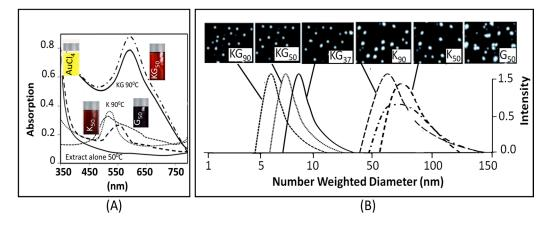
**Figure 3.** Optical absorption curves (**A**); size distribution and transmission electron microscopy (**B**) of different AuNP preparations. Abbreviations: K: kudzu, G: gum, and 37, 50, and 90: reaction temperature in  $^{\circ}$ C.
