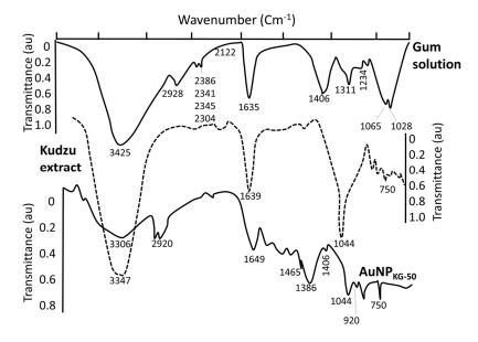
Figure 2. Typical FTIR spectra for AuNP<sub>KG</sub>, kudzu extracts, and gum solution.
