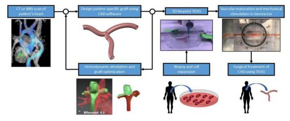
**Figure 15.** Proposed workflow of patient-specific TEVG fabrication. CAD-computer aided design, TEVG—tissue engineered vascular grafts. Reprinted with permission from Lee et al. [107].
