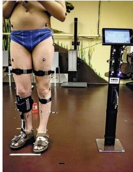
**Figure 5.** Examination in the Laboratory for Movement Analysis of the University of Basel Children’s Hospital (UKBB), Basel, with MOWA—orthosis and simultaneous gait analysis with MOWA inertial sensors.
