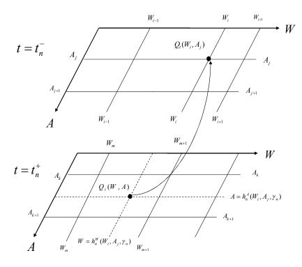
**Figure 1.** Illustration of the application of jump condition. The value  $Q_t(W_i, A_j)$  at  $t = t_n^-$  and at the node point  $(W_i, A_j)$  equals to  $Q_t(W, A)$  at  $t = t_n^+$  with  $W = h_n^W(W_i, A_j, \gamma_n)$  and  $A = h_n^A(W_i, A_j, \gamma_n)$ . The point (W, A) is located inside the grid bounded by  $(W_m, W_{m+1})$  and  $(A_k, A_{k+1})$ .
