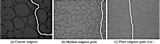
(a) Coarser tungsten grain size: intergranular fracture(predominanly interfacial failure) (b) Medium tungsten grair size : intergranular fracture(predominanly matrix failure)
