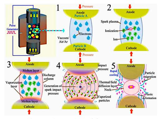
Figure 9. Neck formation mechanism in SPS Process [40].
