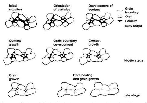
**Figure 14.** Grain growth during the sintering process. (Source: http://www.keramverband.de/brevier\_engl/4/1/4\_1\_4.htm, accessed on 15 September 2022) [68].
