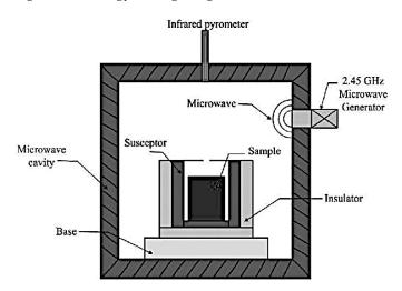
Figure 2. Schematic of microwave sintering furnace [32].
