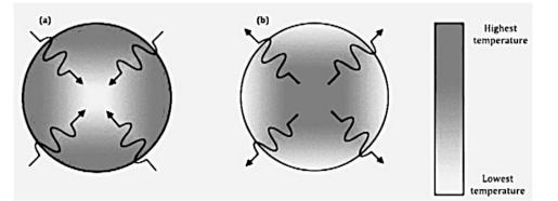
Figure 3. Heating profiles in (a) conventional, (b) microwave [33].
