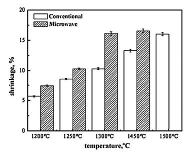
Figure 18. The heating mode impacts radial shrinkage [110].
