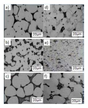
**Figure 19.** Optical image of WHA's (**a**) MA (95W–1.5Fe–3.5Ni), (**b**) MA (93W–1Fe–4.5Ni–1.5Co), (**c**) MA (90W–4Cu–6Ni), (**d**) chemical method (95W–1.5Fe–3.5Ni), (**e**) chemical method (93W–4.5Ni–1Fe–1.5Co), (**f**) chemical method (90W–4Cu–6Ni).
