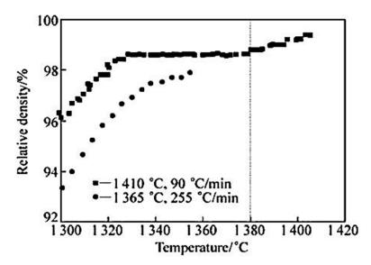
Figure 11. Relative density with sintering temperature [47].
