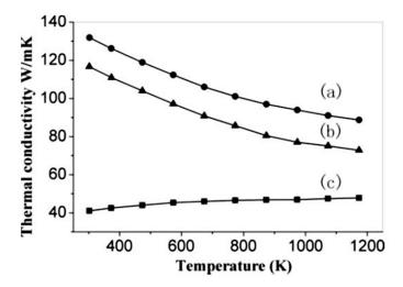
**Figure 7.** Thermal conductivity: (**a**) carbide ball mill W powders (nm), (**b**) carbide ball mill W powders (micron), (**c**) SS-ball milled W powders (micron) [38].
