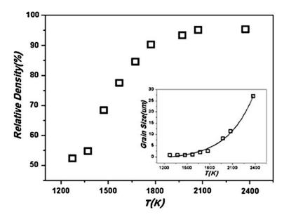
Figure 10. Densification curve of tungsten with various temperatures [44].
