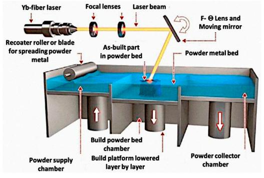
Figure 12. Schematic representation of the L-BPF process [51].
