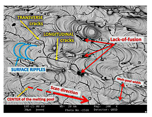
Figure 13. Crack on the tungsten surface in LPBF processed sample [58].
