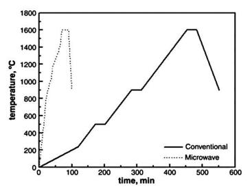
Figure 4. Comparison of the thermal profiles: conventional and microwave [37].
