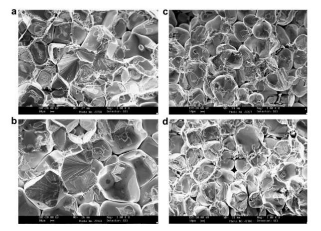
**Figure 15.** SEM fractography images of W–Ni–Cu-heavy alloy [90]. (a) W-94.9, Ni-3.4, Cu-1.7 alloy, (b) W-96.1, Ni-2.8, Cu-1.1 alloy, (c) W-92.5, Ni-5, Cu-2.5 alloy and (d) W-96.0, Ni-2.8, Cu-1.1, Fe-0.1 alloy.
