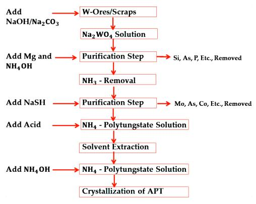
Figure 1. Flow diagram of tungsten hydrometallurgical process [3].
