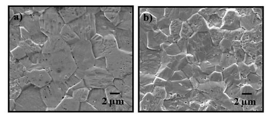
Figure 5. SEM micrographs: (a) conventional sintering and (b) microwave sintering [37].
