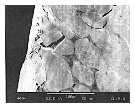
Figure 17. Microcracks at W-W grain boundaries in shear band region [106].
