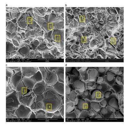
**Figure 20.** Fractography images (**a**) 90W–3Fe–7Ni (MW-sintered), (**b**) 90W–2Fe–6Ni–2Co (MW-sintered), (**c**) 90W–3Fe–7Ni (conventionally sintered), (**d**) 90W–2Fe–6Ni–2Co (conventionally sintered).
