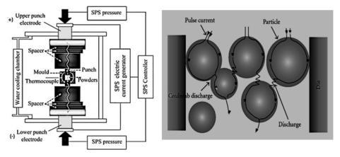
Figure 8. Schematic illustration of the features of SPS [39].
