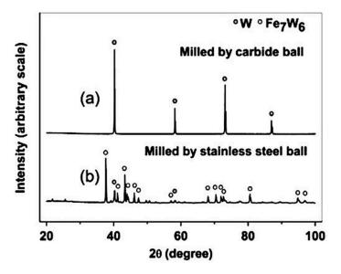
Figure 6. XRD profiles of tungsten by MW process [38].
