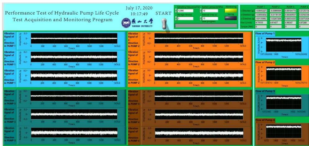
Figure 10. Data acquisition program front panel.
