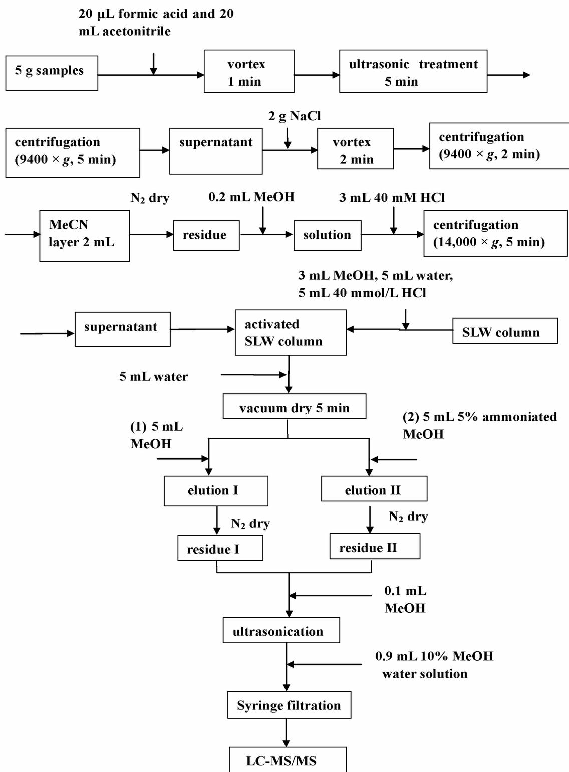
**Figure 6.** Flow chart of the extraction and purification processes of PGRs in samples.
