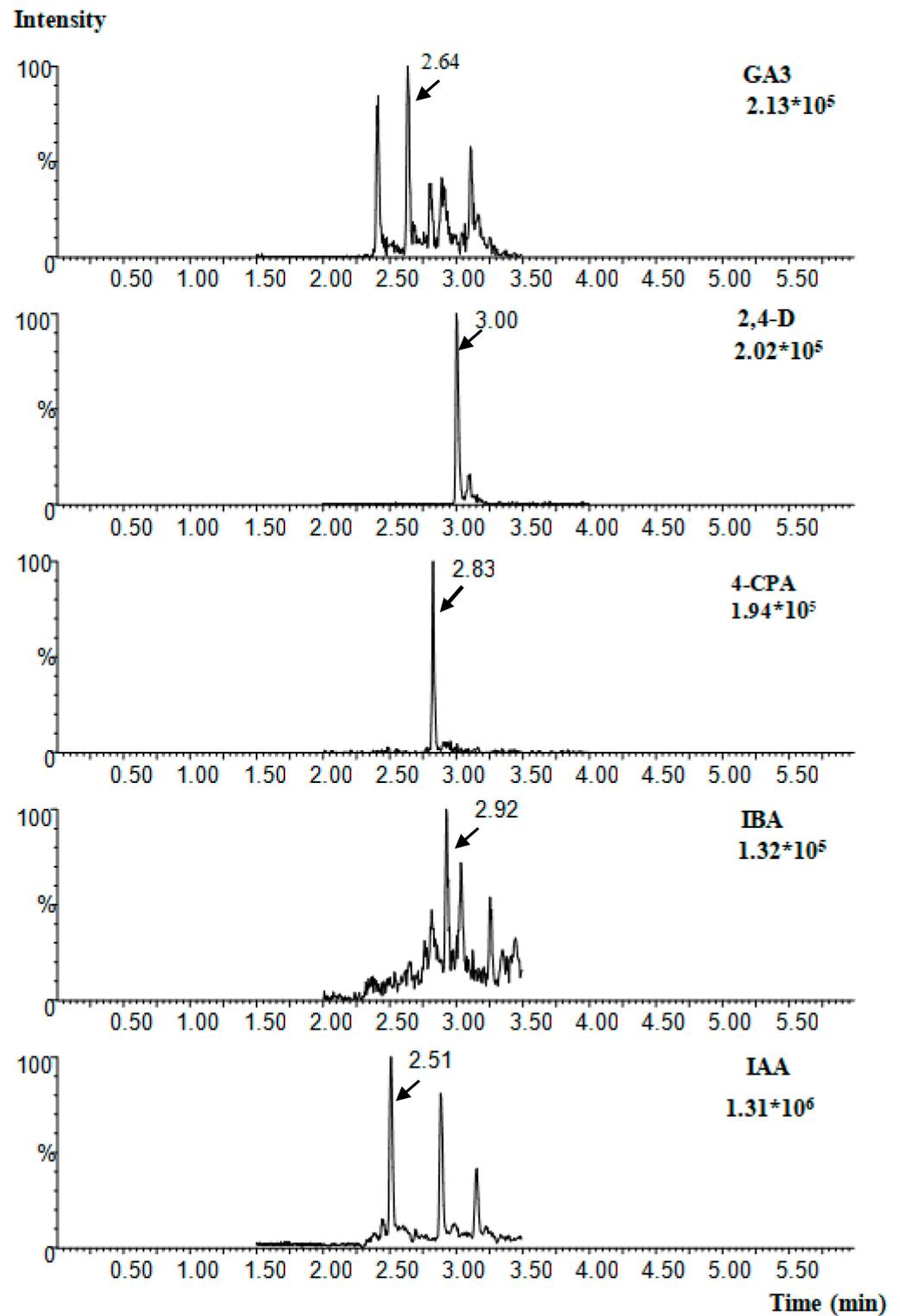
**Figure 4.** EICs of the five PGRs present in elution I from sample 1 after the addition of 5 ng/g standard solutions.
