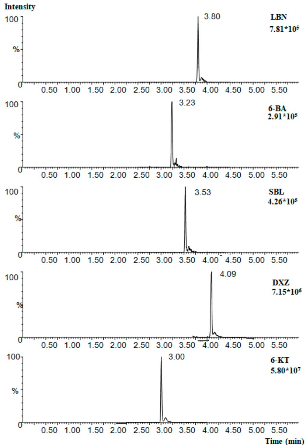
**Figure 5.** EICs of the five PGRs present in elution II from sample 1 after the addition of 5 ng/g standard solutions.
