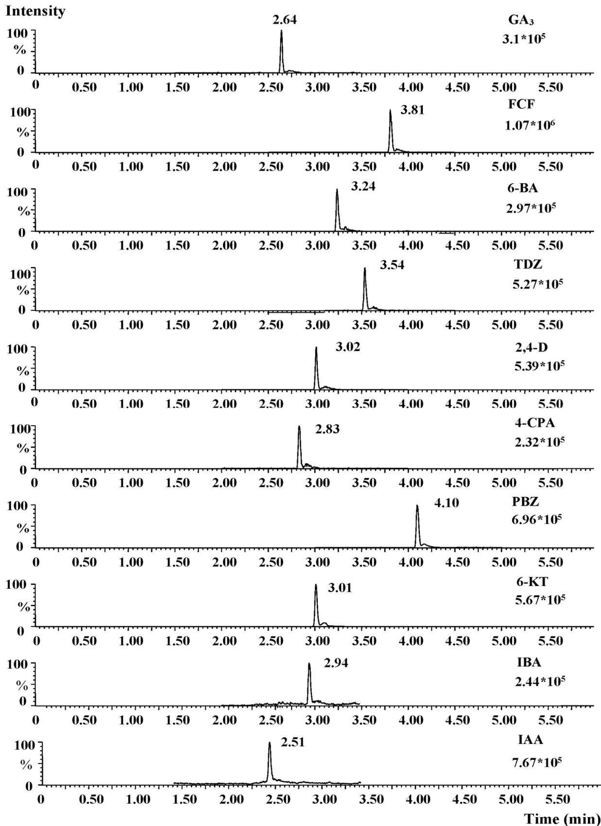
**Figure 1.** Total ion chromatogram of the 10 PGR standard solutions. Numbers under the PGRs indicate the signal intensity.
