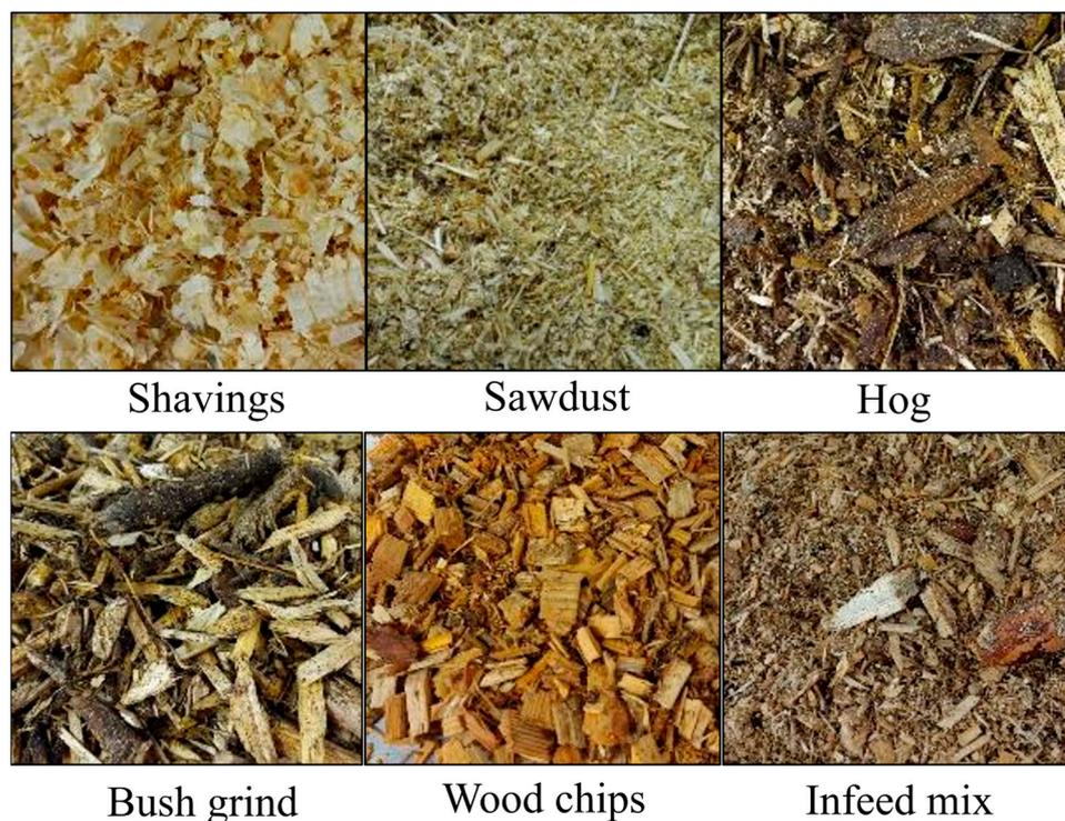
**Figure 1.** Images of the six groups of infeed materials tested in this paper. This image was previously published in Canadian Biomass Magazine [14].
