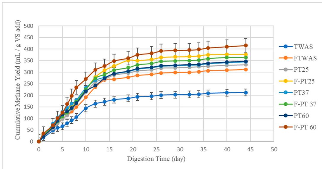
**Figure 8.** Cumulative methane production ( $\text{mL/g VS added}$ ) comparison between FNA-Heat pretreated and/or Fermented samples and the raw TWAS. Error bars are shown only for the control and the sample with the highest cumulative methane yield (i.e., F-PT-60), with omitted bars for other samples as errors were less than 5%, enhancing figure clarity.
