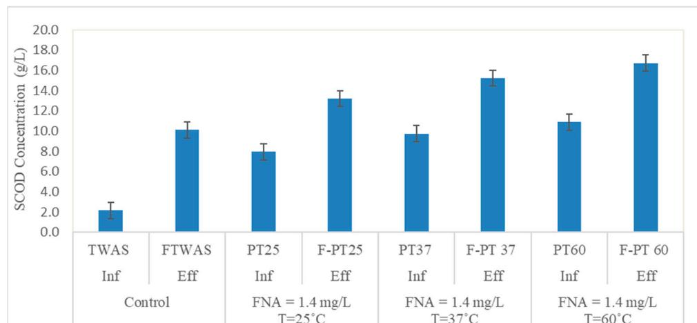
**Figure 5.** SCOD concentration (g/L) in the fermented, FNA-heat pretreated, and raw TWAS (error bars represent the standard errors).
