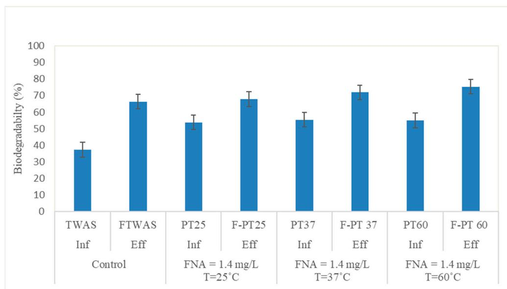
**Figure 9.** Biodegradability of FNA-Heat pretreated/fermented samples compared to the raw TWAS (error bars represent the standard errors).
