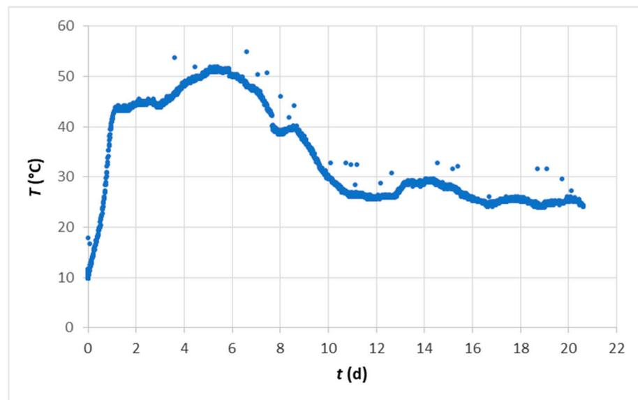
**Figure 1.** Temperatures measured during the experiment on the aerobic stabilization of biowaste in the reactor.
