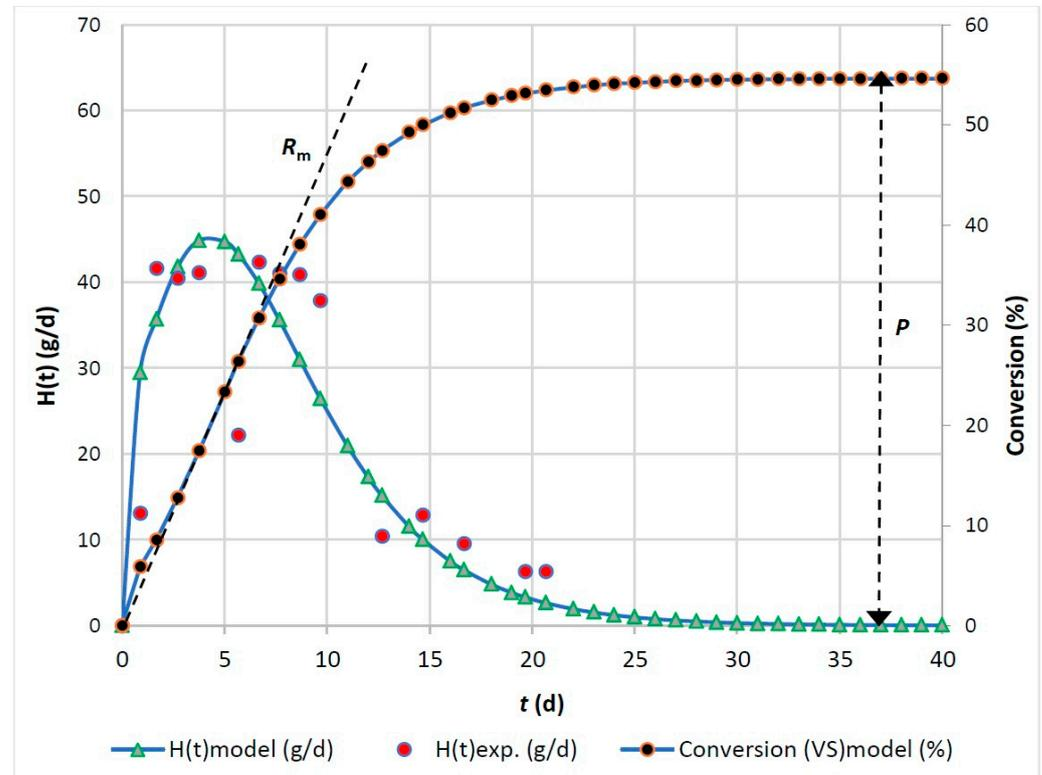
**Figure 3.** Simulation of CO<sub>2</sub> formation and conversion of biodegradable VS in the process of aerobic biodegradation of a biowaste sample.
