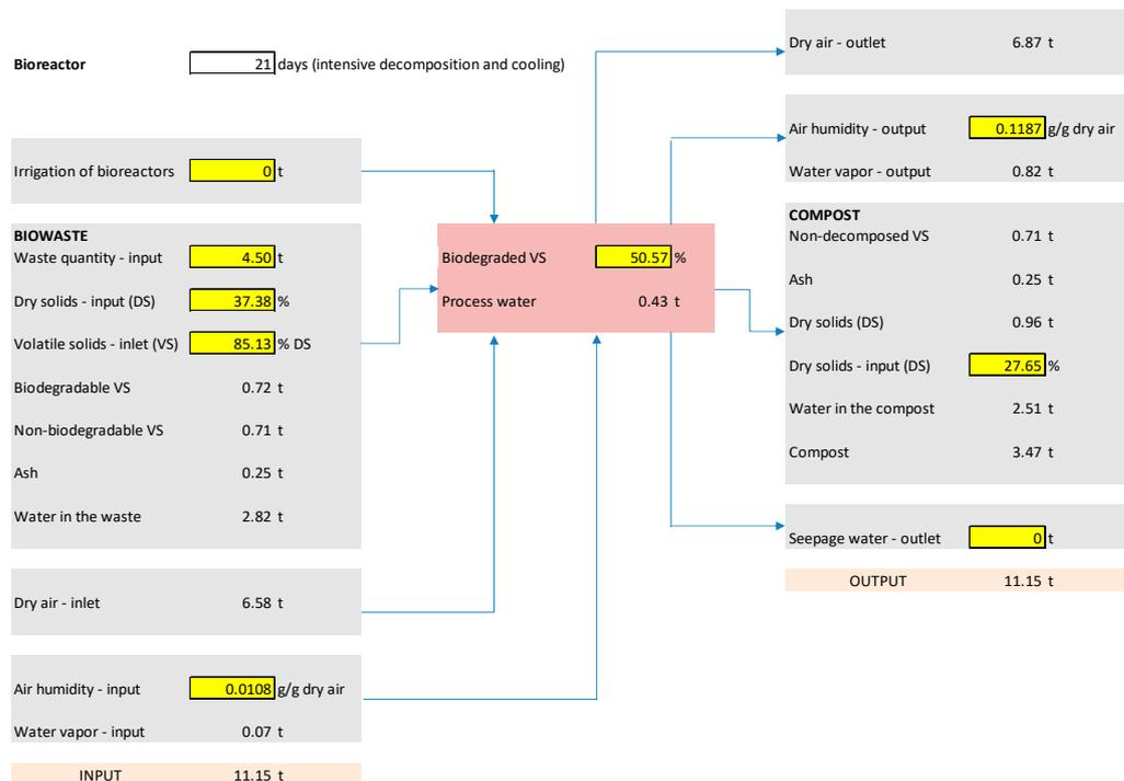
**Figure 2.** Mass balance of the aerobic biodegradation process of a biowaste sample (Excel worksheet screenshot).
