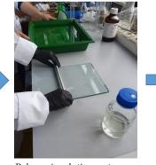
Polymeric solution cast on a flat glass sheet using a "doctor blade" device
