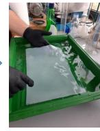
Casted membrane immersed within ultrapure water coagulation bath
