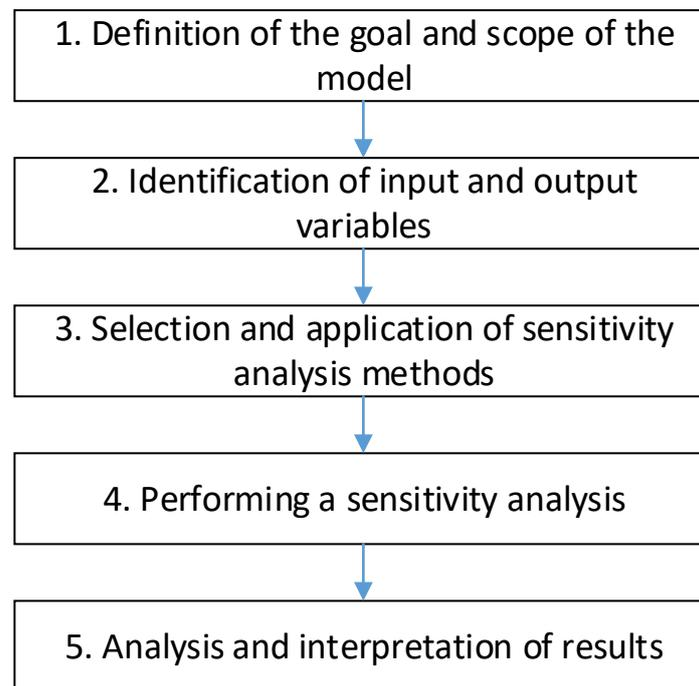
**Figure 3.** Stepwise algorithm for sensitivity analysis.
