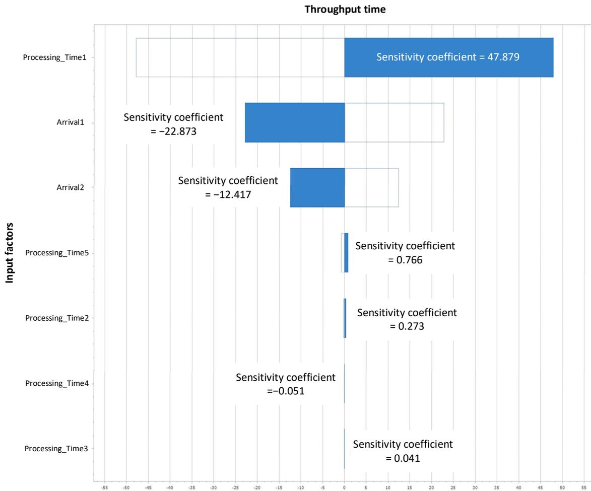
**Figure 8.** Tornado sensitivity analysis graph for throughput time.
