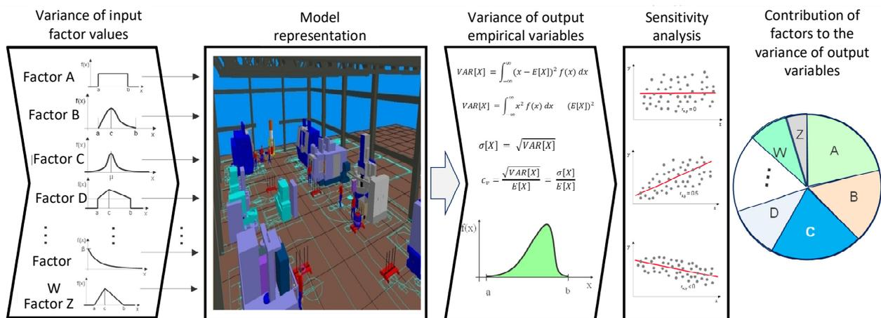
Figure 1. The principle of global sensitivity analysis.
