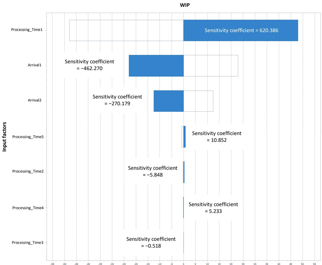
**Figure 9.** Tornado chart for production in progress.
