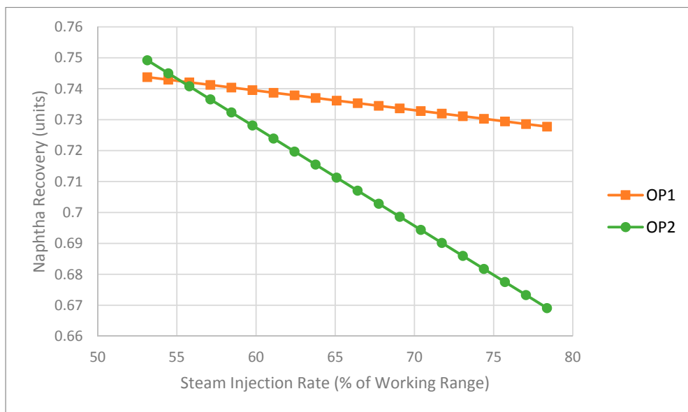
Figure 7. Impact of steam injection rate on naphtha recovery (NR) as predicted by statistical models ( NF = 0.863 wt.%, F_{feed} = 4247 bbl/h).
