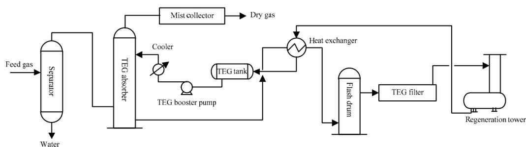
**Figure 1.** Conventional triethylene glycol (TEG) dehydration process.
