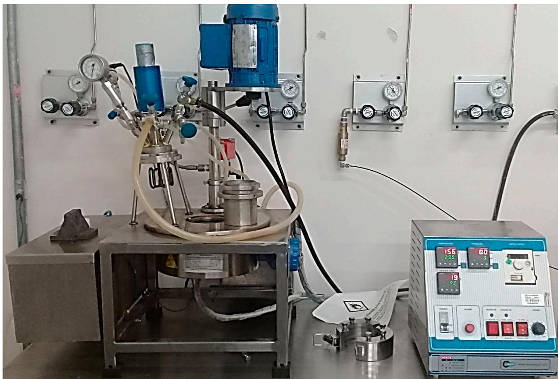
Figure 1. Stirred tank batch reactor.
