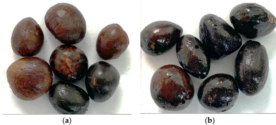
**Figure 6.** Picture of palm kernel before ((a): 0.28 kg/kg) and after ((b): 0.07 kg/kg) the drying process at 80 °C.
