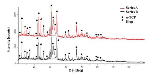
Figure 3. XRD patterns of the biomicroconcretes.
