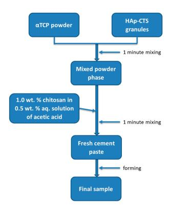
**Figure 2.** The flow chart of the preparation procedure.
