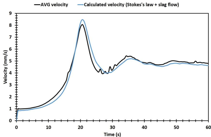
Figure 7. Average velocity of droplets and calculated velocity.
