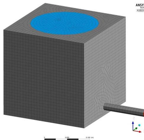
**Figure 3.** Geometry and mesh of the CFD model for CFD-DEM simulation. Inlet (blue) on the top and tapping hole (red) on the right side.
