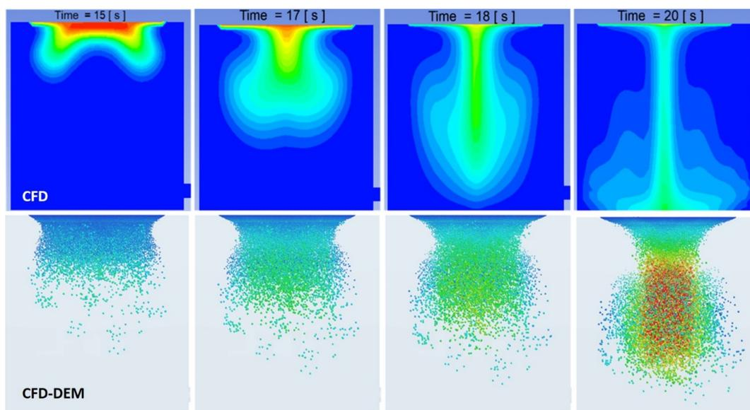
**Figure 10.** A comparison of the CFD and CFD–DEM results for matte settling in the small-scale settler model, revealing a similar funneling flow pattern at 15, 17, 18, and 20 s. Upper row: CFD, lower row: CFD–DEM.
