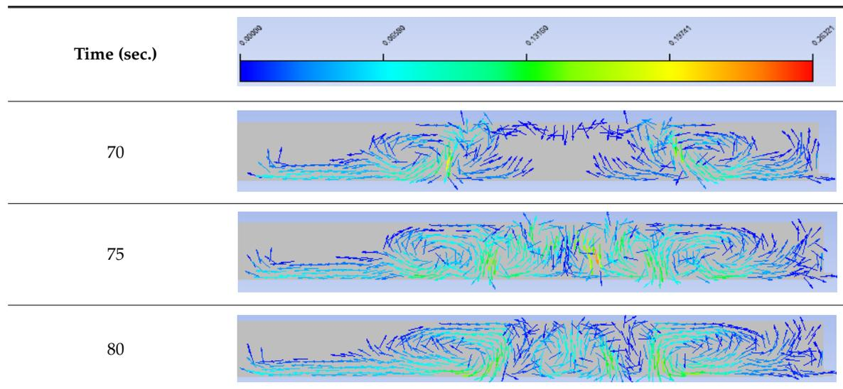
Finally, when we compare the volume fraction contours of the smaller-sized settler presented in Table 4, and the volume fraction contours of the full-size settler presented in Table 6, we can observe a significant difference. This is because in the full-size settler instead of a single funnel-shaped flow, different locally channelled flows are formed, which is exhibited in the profile. The same phenomenon is depicted in the velocity vector profiles in Tables 5 and 7.
