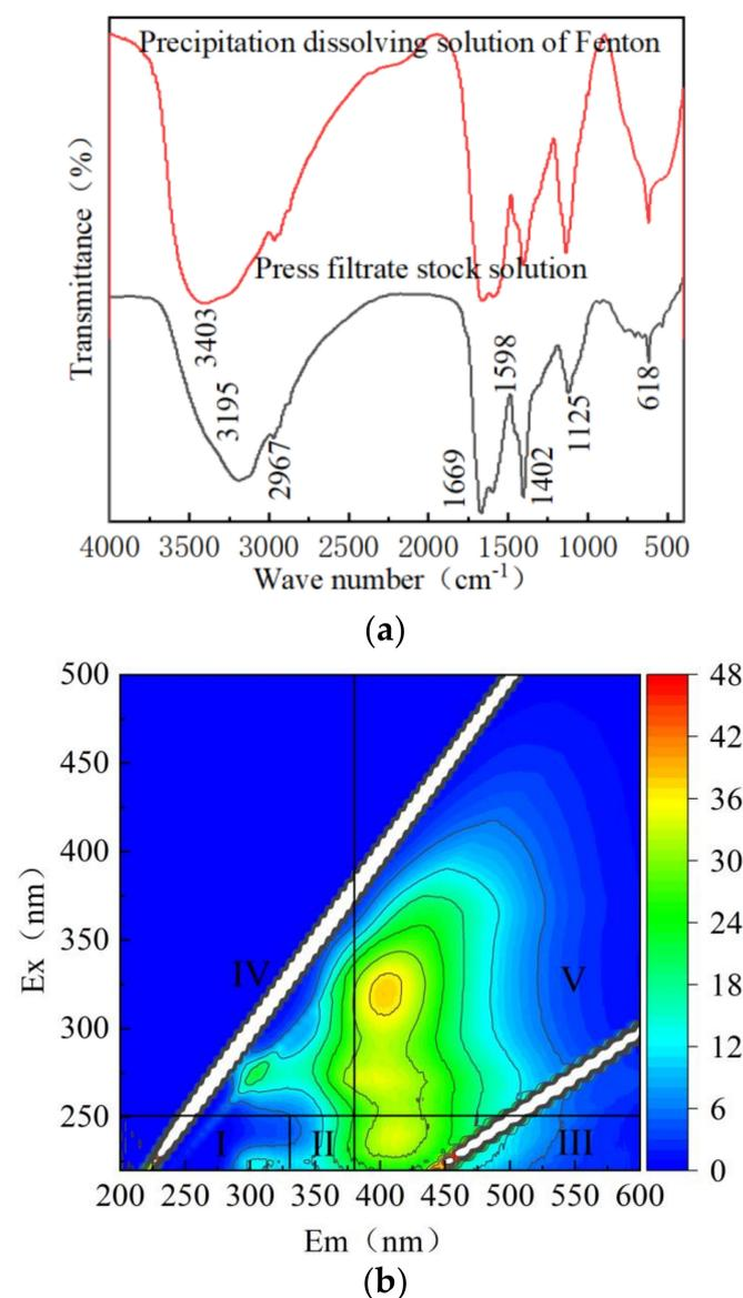
Figure 8. Fenton precipitate solution: (a) FTIR diagram, (b) three-dimensional fluorescence.
