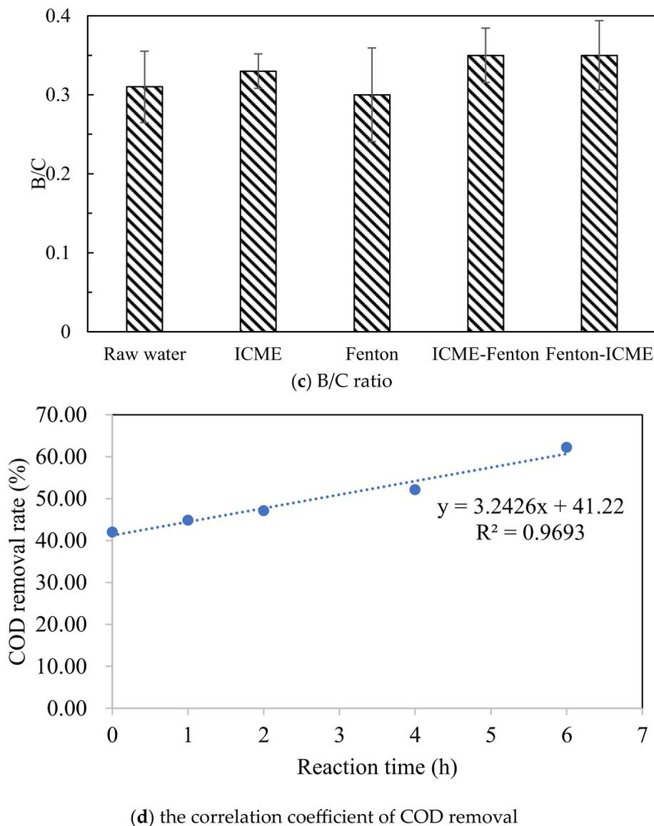
**Figure 5.** The performance comparison of different process: (a) COD removal, (b) effluent color, (c) B/C ratio, (d) the correlation coefficient of COD removal.
