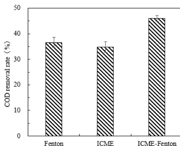
**Figure 2.** The COD removal via Fenton oxidation, ICME, and ICME-Fenton process.
