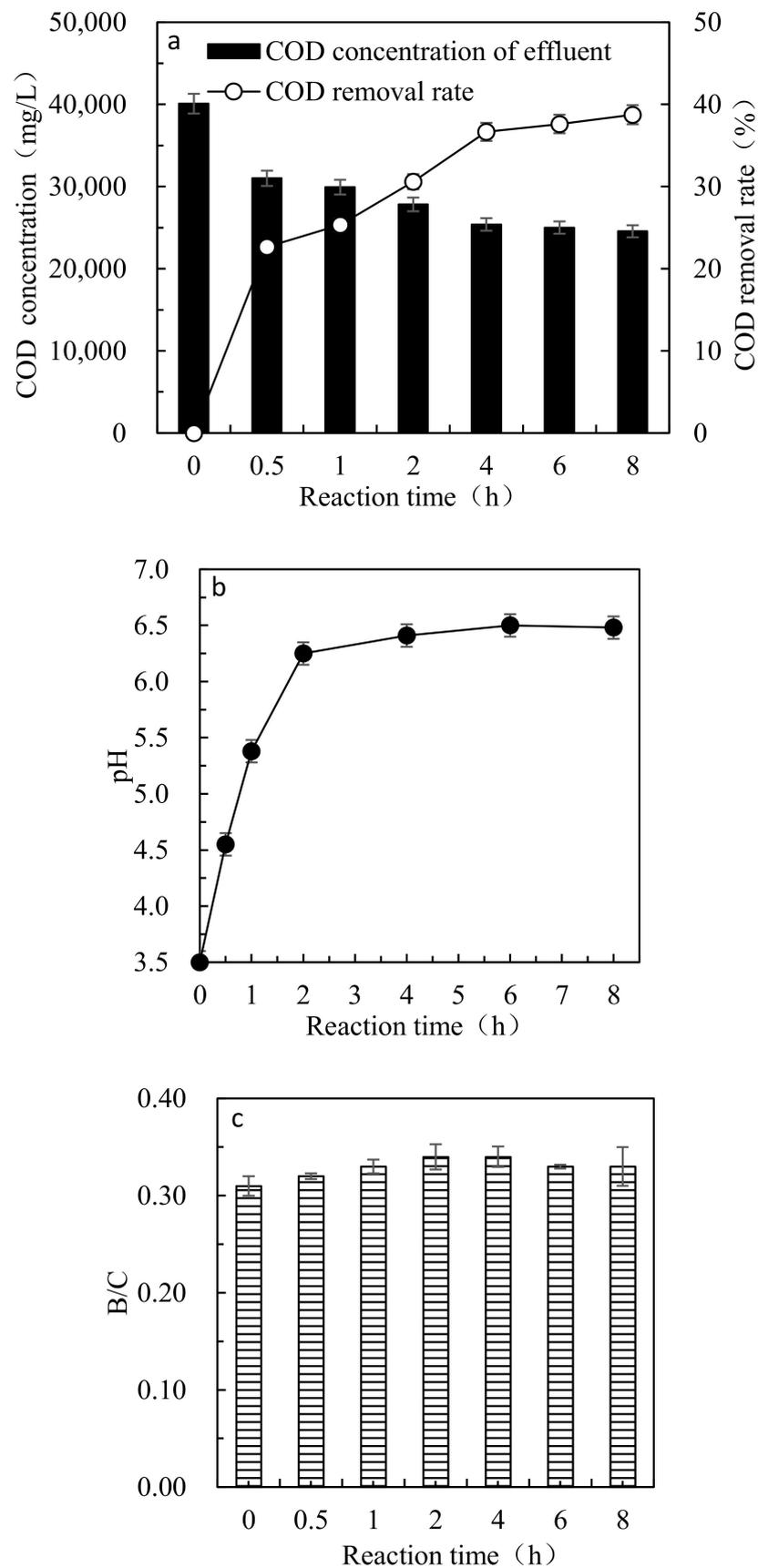
**Figure 1.** The COD removal (a), pH variation (b), and the ratio of BOD to COD (c) of leachate before and after ICME treatment.
