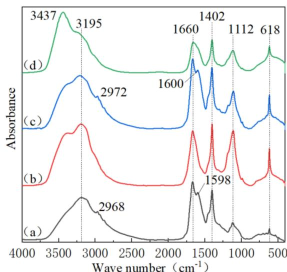
**Figure 6.** FTIR spectra of filtrate and effluent: (a) original leachate; (b) Fenton-treated; (c) ICME-treated; (d) Fenton-ICME-treated.
