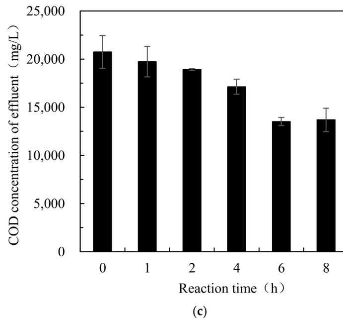
**Figure 4.** Effect of relevant parameters on COD removal of the leachate via the Fenton-ICME combined process: (a) pH value, (b) the filler dosage, (c) reaction time.
