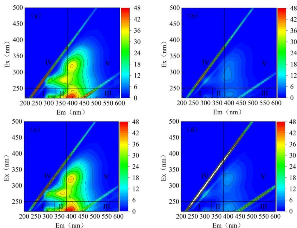
**Figure 7.** Three-dimensional fluorescence images of the leachates: (a) original leachate, (b) treated with Fenton oxidation, (c) treated with ICME, (d) treated with the Fenton-ICME process.
