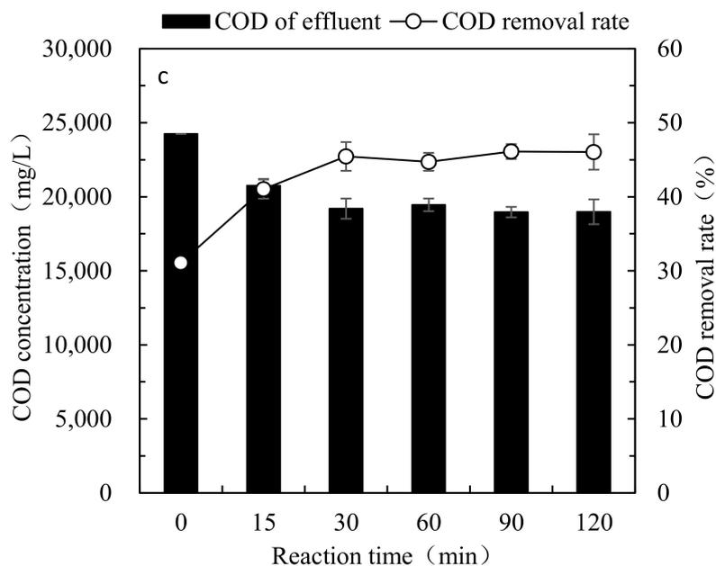
**Figure 3.** Effect of relevant parameters on COD removal from leachate via the ICME-Fenton combined process: (a) H<sub>2</sub>O<sub>2</sub> dosage, (b) pH, (c) reaction time.
