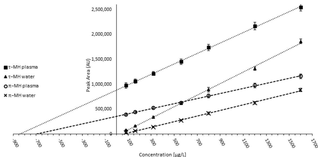
**Figure 4.** Standard addition and surrogate matrix calibration curves for  $\tau$ - and  $\pi$ -methylhistidine at the selected concentrations. Extrapolation of the standard addition curve indicates the endogenous value of  $\tau$ - and  $\pi$ -MH in the pooled sample.
