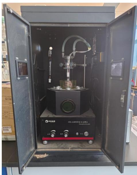
**Figure 1.** Photochemical reaction system.
