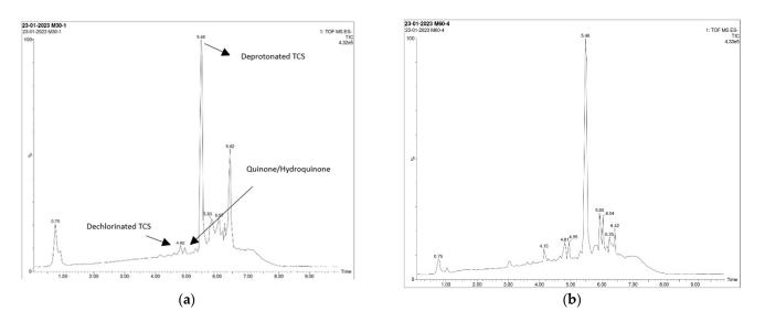
Figure 7. HPLC chromatograms of TCS irradiated with simulated solar light for (a) 30 min and (b) 4 h.
