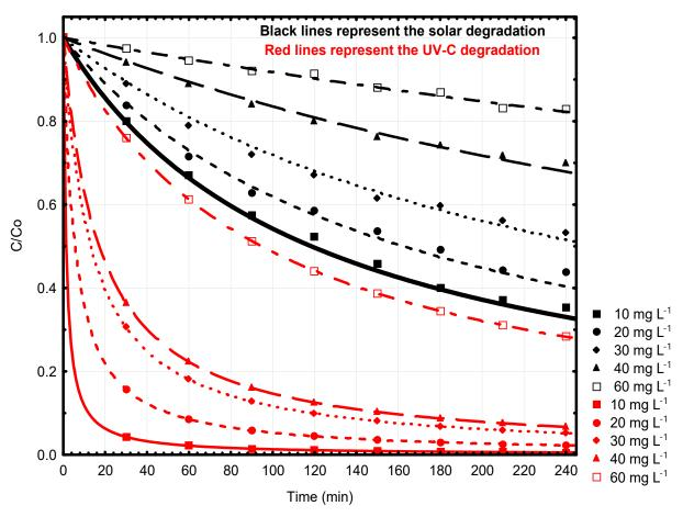
UV-C light. To enhance the process efficiency, small amounts of radicals, like potassium persulphate, can be added to the photoreaction solution [26].
