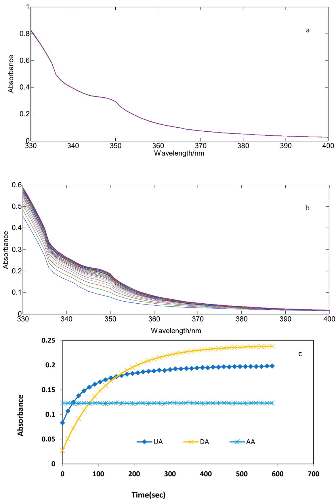
**Figure 1.** Spectrophotometric spectra of (a) UA, (b) DA and (c) Kinetic profiles of DA, UA and AA at acetate media (pH = 4.5) and wavelength 320 nm.
