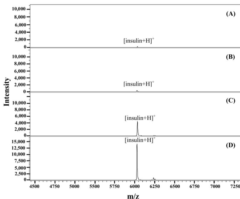
**Figure 2.** Mass spectra of insulin obtained with different membranes: (A) PVDF, (B) PTFE, (C) MCE, and (D) nylon. Experimental conditions: insulin volume, 3  $\mu$ L; SA solution volume, 3  $\mu$ L; and insulin concentration, 5.0  $\mu$ M. The mass spectrum was obtained by averaging 200 mass spectra using laser energy that slightly exceeded the threshold.
