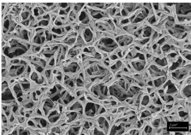
**Figure 3.** SEM image of the nylon membrane. The SEM operated at an accelerating voltage of 20 kV.
