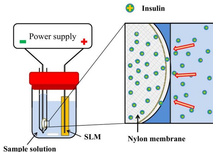
**Figure 1.** Schematic illustration of the EME setup.
