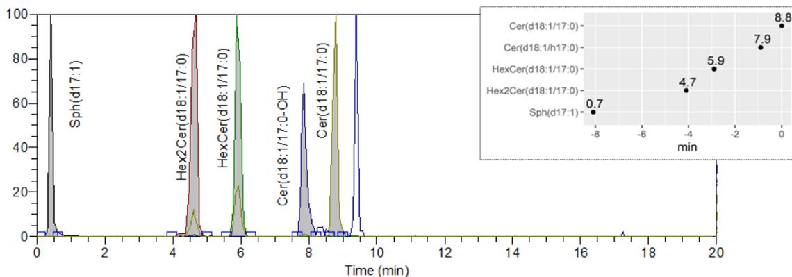
**Figure 1.** Annotated LC-MS/MS chromatogram for internal standards used for the method development of ceramides and glycosceramides analysis. The inset image presents retention time variations due to the structural differences, i.e., sequential addition of hexoses and hydroxylation of the fatty acyl chain, as well as the free sphingoid base retention time.
