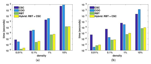
**Figure 6.** Wall-clock time taken to insert elements into a  $10,000 \times 10,000$  sparse matrix to achieve various densities of non-zero elements. In (a), the elements are inserted at random locations in random order. In (b), the elements are inserted in a quasi-ordered fashion, where each new inserted element is at a random location that is past the previously inserted element, using column-major ordering.
