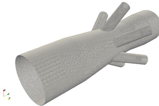
Figure 13. Boundary particles of the discretized geometry for the cylindrical nozzle case.
