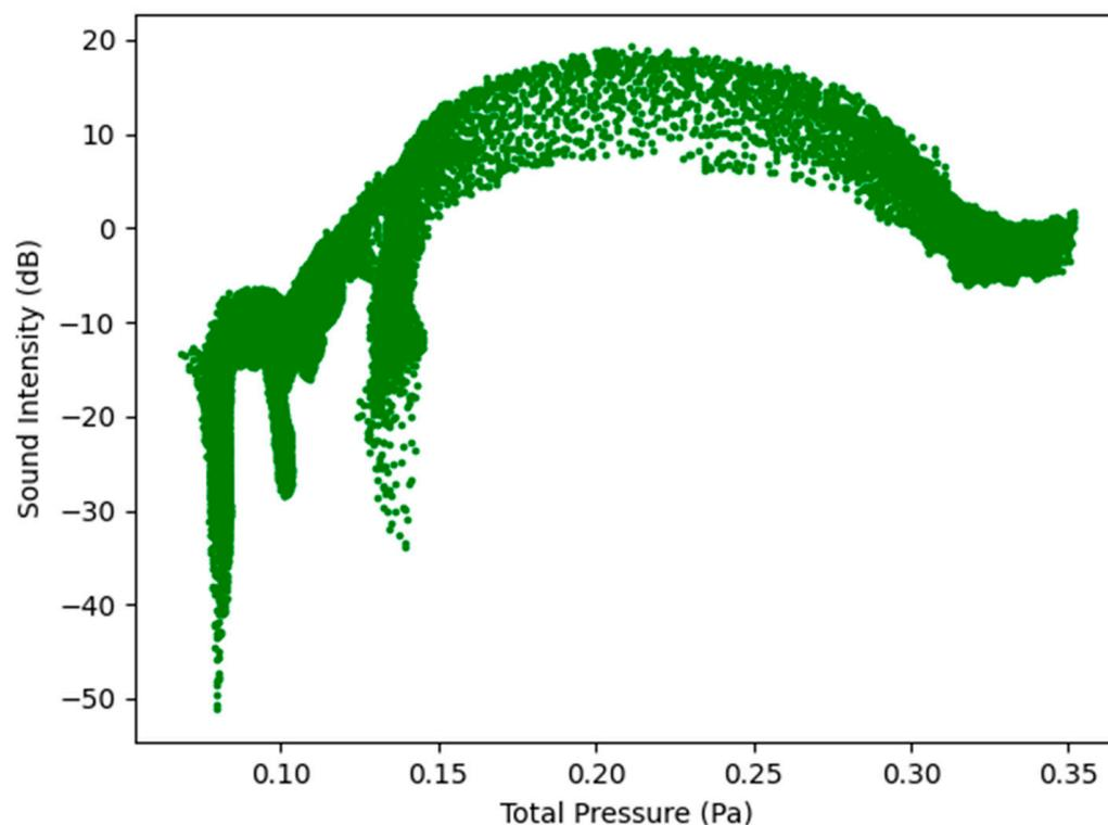
Figure 11. Sound Intensity as a function of Total Pressure at 7.5 L/s—Healthy Lungs.
