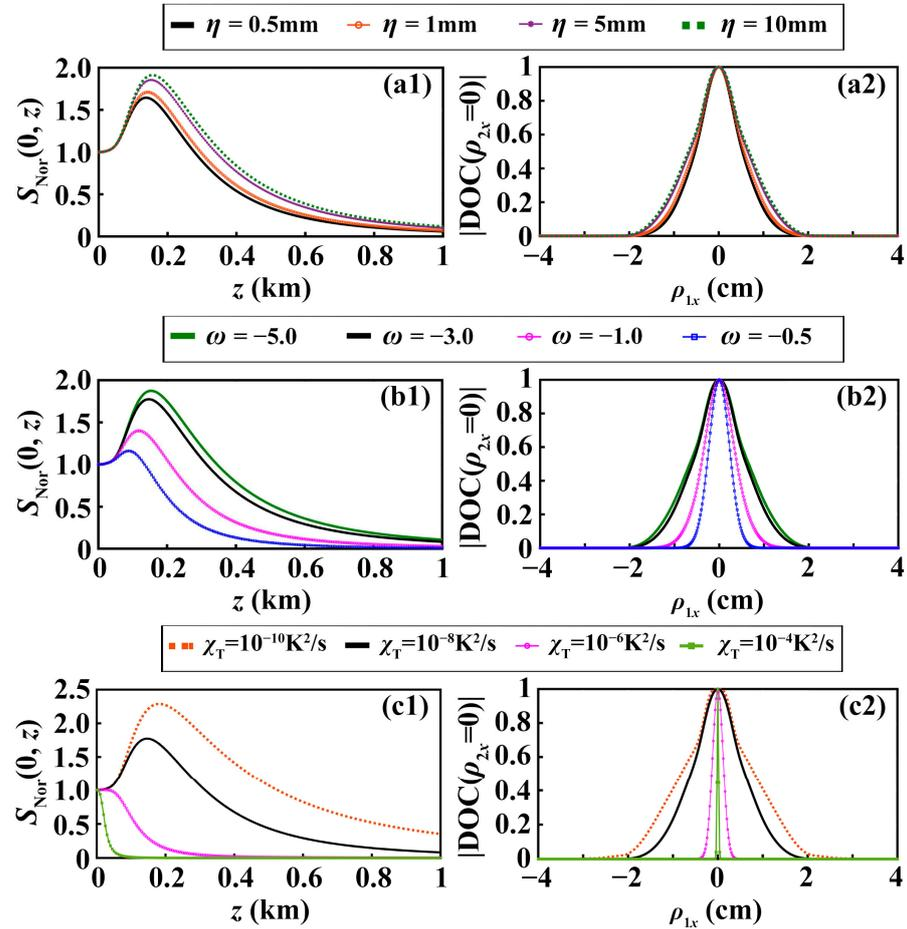
**Figure 7.** Normalized on-axis intensity of the LNUC beam propagating in oceanic turbulence and the cross-line ( $\rho_{2x} = 0$ ) of the absolute value of the spectral DOC at  $z = 150$  m for different oceanic turbulence parameters: (a) the Kolmogorov inner scale; (b) the relative strength of temperature to salinity undulations; (c) the dissipation rate of mean-square temperature.
