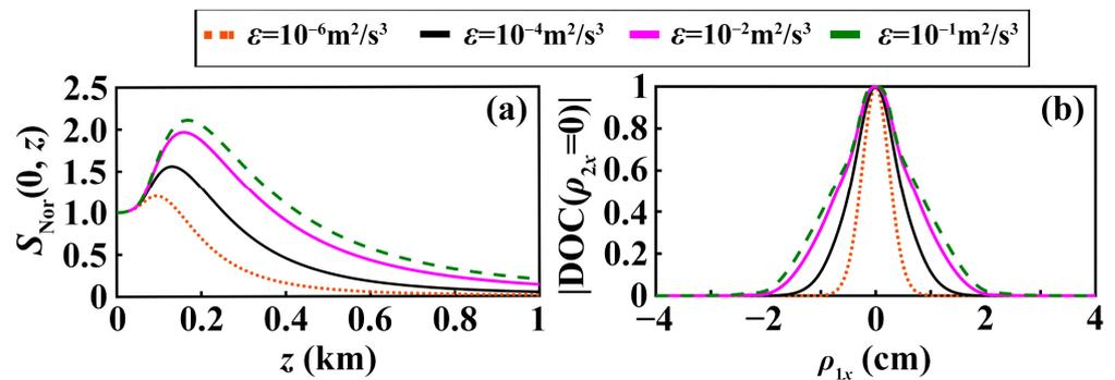
**Figure 6.** (a) Normalized on-axis intensity of LNUC beams propagating in oceanic turbulence and (b) the cross-line ( $\rho_{2x} = 0$ ) of the absolute value of the spectral DOC at  $z = 150$  m for different rates of dissipation of kinetic energy per unit mass of fluid.
