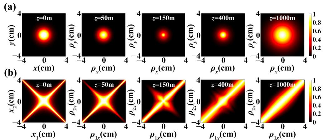
Figure 4. Evolution of the (a) normalized spectral intensity and (b) spectral DOC on propagation in oceanic turbulence.
