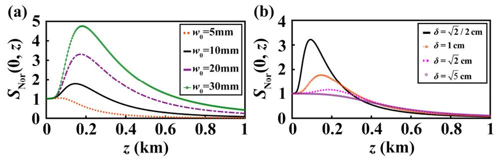
**Figure 8.** Normalized on-axis intensity of LNUC beams propagating in oceanic turbulence for different (a) beam widths and (b) coherence lengths.
