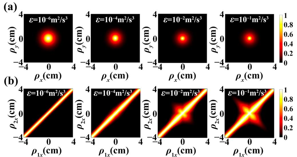
**Figure 5.** Density plot of (a) the normalized spectral intensity and (b) the absolute value of the spectral DOC of a LNUC beam in oceanic turbulence with different values of the dissipation rate of kinetic energy per unit mass of fluid at propagation distance  $z = 150$  m.
