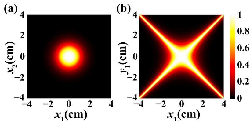
**Figure 1.** Density plot of the absolute value of the spectral DOC of a LNUC beam (a) in the  $x_1 - x_2$  plane with  $y_1 = y_2 = 0$ , (b) in the  $x_1 - y_1$  plane with  $x_2 = y_2 = 0$ .
