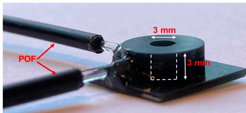
**Figure 5.** Image of the fabricated sensing assay compartment. The dashed line indicates the compartment.
