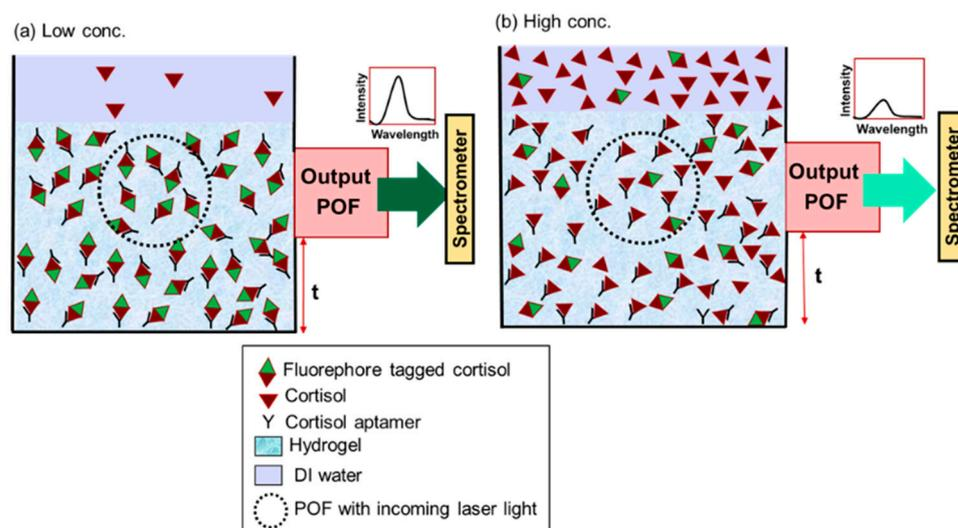
**Figure 1.** Schematic diagram of the sensing principle: (a) low cortisol concentration; (b) high cortisol concentration. (The dotted circle indicates the POF with incoming light;  $t$  is the distance between the bottom of the assay compartment and the fibers.)
