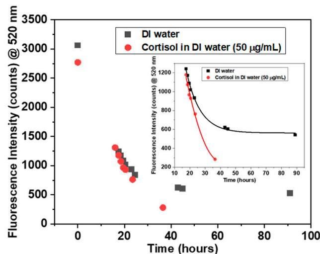
Figure 7. Fluorescence intensity vs. time with exposure to cortisol (50  $\mu\text{g}/\text{mL}$ ) solution. The inset shows the fluorescence intensity vs. time from 20 h to 90 h.
