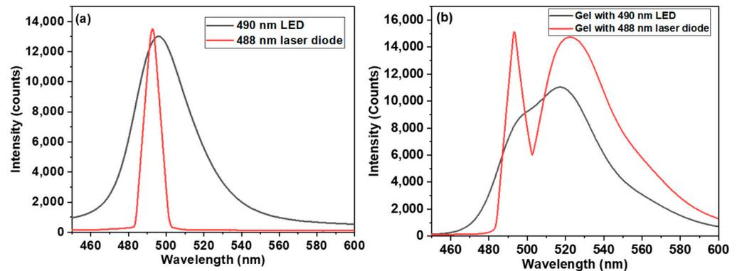
**Figure 4.** (a) The output spectra of the 490 nm LED and 488 nm laser diode. (b) The spectra of the 490 nm LED and 488 nm laser diode together with AF488H fluorescence after passing through the C3CMO-AF488H-containing hydrogel.
